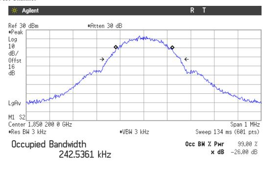
Transmit Freq Error 1.305 kHz x dB Bandwidth 312.719 kHz
