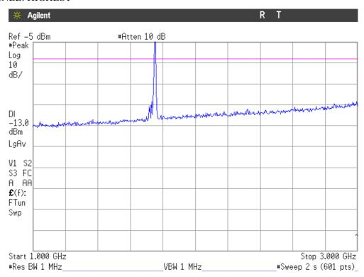
Note: The peak above the limit is the carrier frequency.
