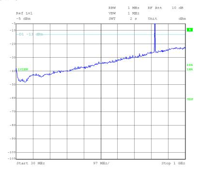
Note: The peak above the limit is the carrier frequency.
