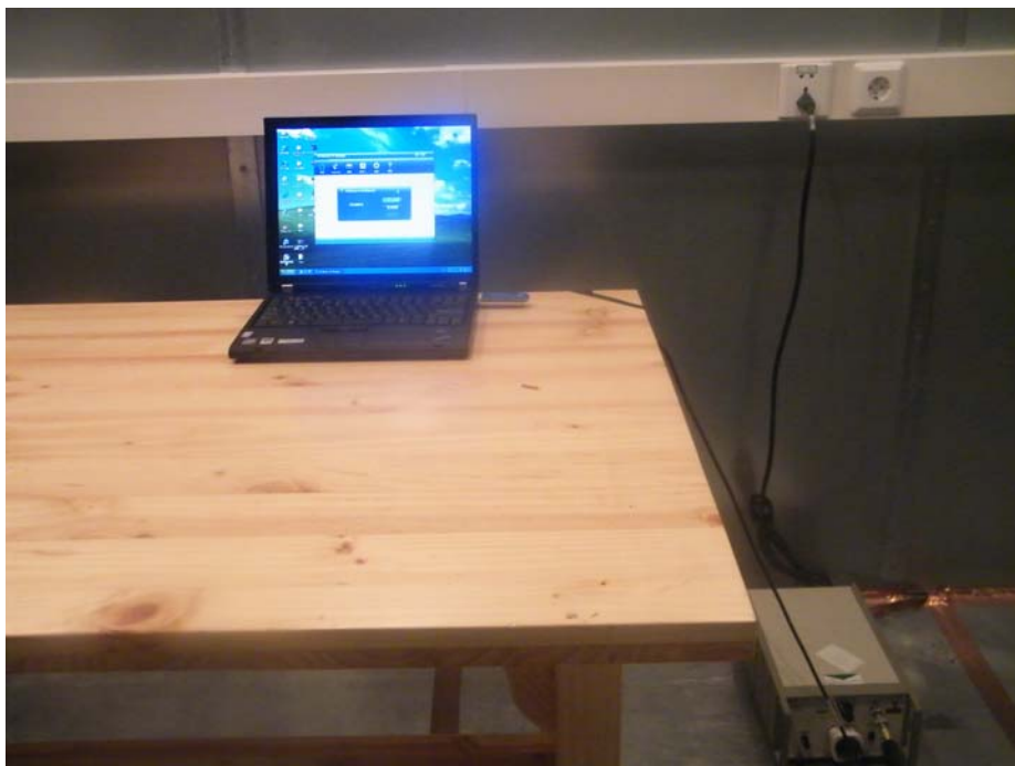
Picture 3 Conducted Emission Test Setup
