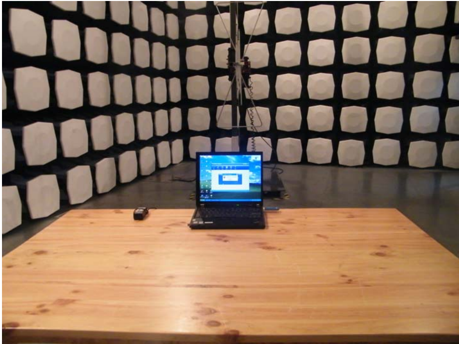
Picture 2 Radiated Emission Test Setup
