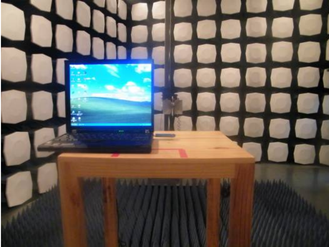
Picture 2: Radiated Spurious Emissions Test setup
