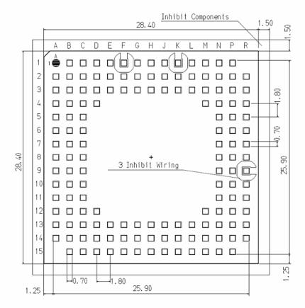
In order to easily rework the ME910C1 is suggested to consider on the application a 1.5 mm placement inhibit area around the module.
