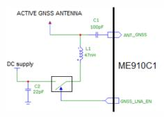
Be aware of max bias current in case of unwanted short on antenna cable, decoupling inductor may be demaged.
