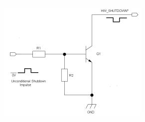
For example: Let us assume you need to drive the HW\_SHUTDOWN\* pad with a totem pole output of a +3/5 V microcontroller (uP\_OUT2):
