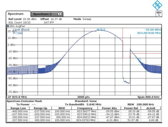
NBIoT BAND 26 (12 Tones 15 kHz.  $\pi/4$  - QPSK Offset 0 MODULATION) Highest Channel:
