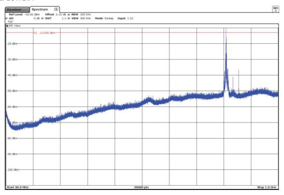
Note: The peak above the limit is the carrier frequency. The peak at 859MHz corresponds to the downlink signal
