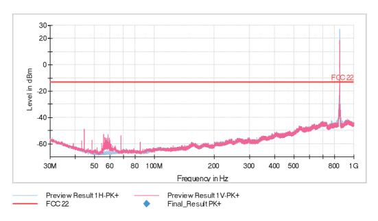
Note: The peak above the limit is the carrier frequency.
