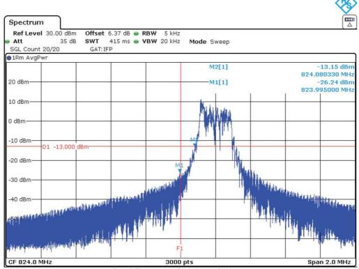
NBIoT BAND 5 (Tone 3.75 kHz. π/2 - BPSK Offset 47 MODULATION)
