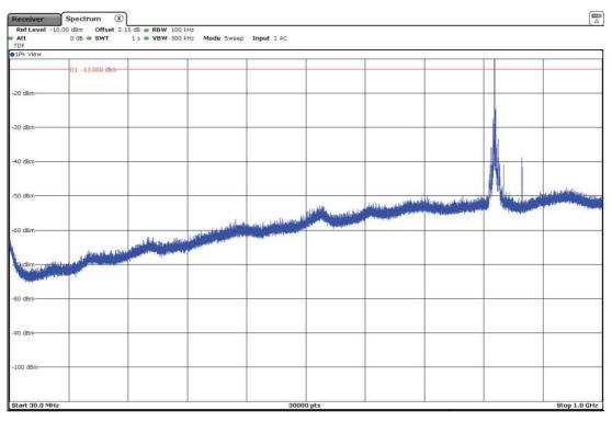
Note: The peak above the limit is the carrier frequency. The peak at 869MHz corresponds to the downlink signal
