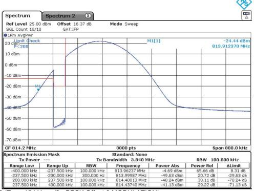
NBIoT BAND 26 (Tone 15 kHz. π/2 - BPSK Offset 0 MODULATION)
