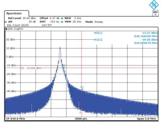
NBIoT BAND 5 (12 Tones 15 kHz.  $\pi/4$  - QPSK Offset 0 MODULATION)
