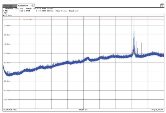
Note: The peak above the limit is the carrier frequency. The peak at 864MHz corresponds to the downlink signal
