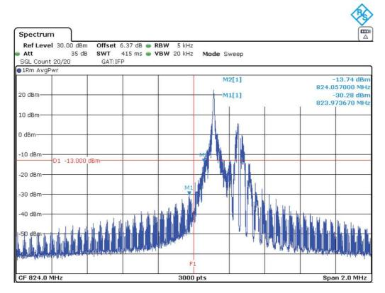
NBIoT BAND 5 (Tone 15 kHz. π/4 - QPSK Offset 0 MODULATION)
