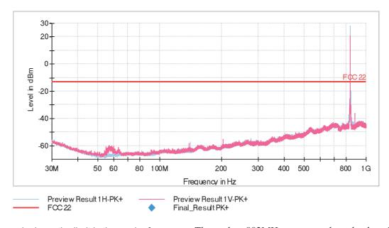
Note: The peak above the limit is the carrier frequency. The peak at 882MHz corresponds to the downlink signal
