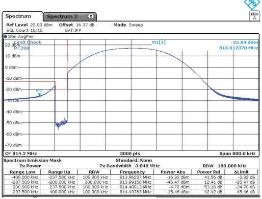
NBIoT BAND 26 (Tone 3.75 kHz.  $\pi/2$  - BPSK Offset 47 MODULATION) Highest Channel:
