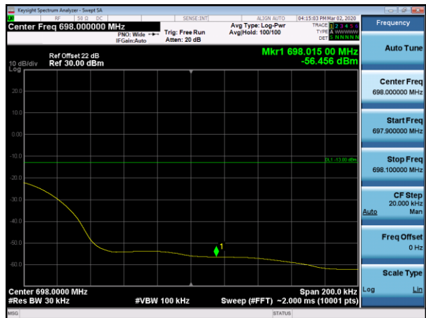
Channel 133470-1 tone offset 47, BW 3.75kHz, QPSK
