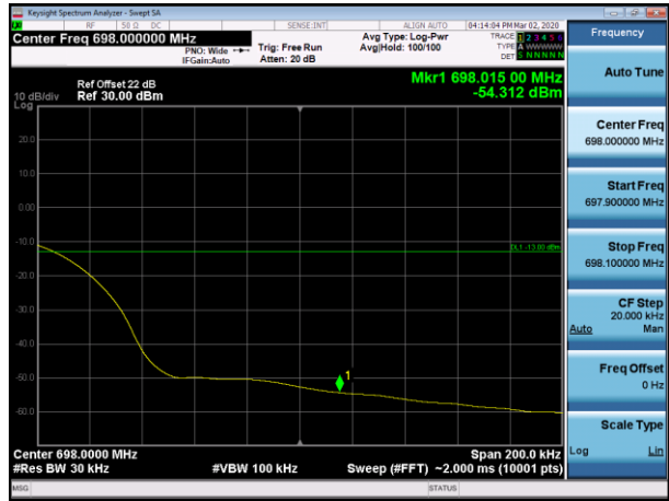
Channel 133470-1 tone offset 47, BW 3.75kHz, QPSK
