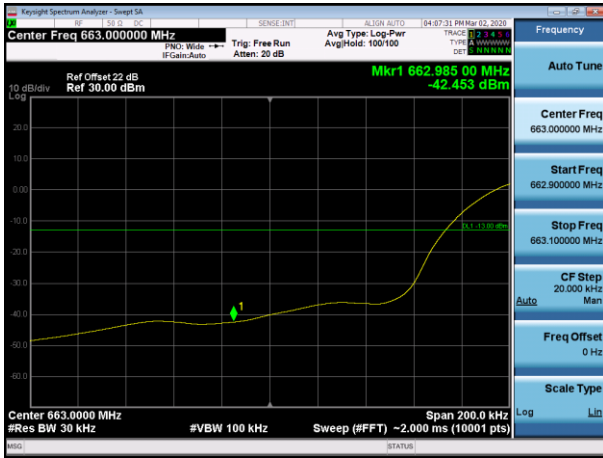
Channel 133124-1 tone offset 0, BW 3.75kHz, QPSK
