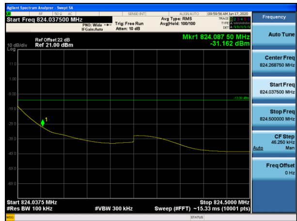
Channel 26788-1 tone offset 47, BW 3.75kHz, QPSK Frequency up to and including 37.5kHz
