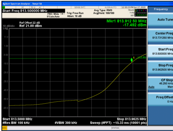
Channel 26691-1 tone offset 0, BW 15kHz, QPSK Frequency up to and including 37.5kHz
