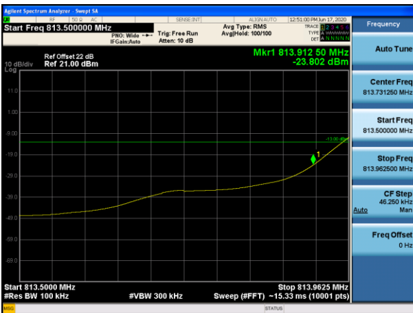
Channel 26691-1 tone offset 0, BW 3.75kHz, BPSK Frequency up to and including 37.5kHz
