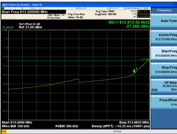
Channel 26692-1 tone offset 0, BW 15kHz, BPSK Frequency greater 37.5kHz
