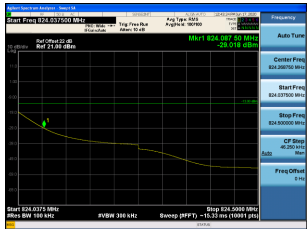
Channel 26788-1 tone offset 11, BW 15kHz, BPSK Frequency greater 37.5kHz
