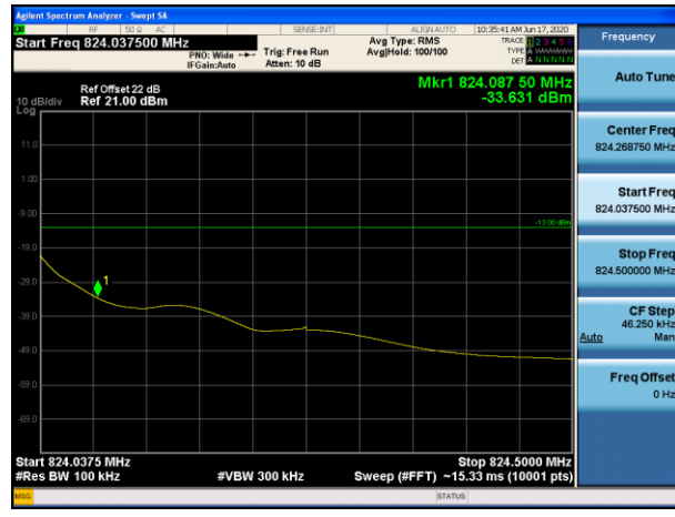
Channel 26788-1 tone offset 47, BW 3.75kHz, QPSK Frequency greater 37.5kHz
