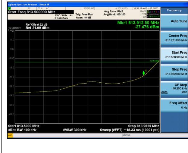
Channel 26692-1 tone offset 0, BW 3.75kHz, QPSK Frequency greater 37.5kHz
