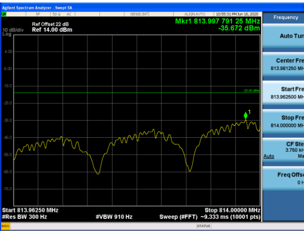
Channel 26691-1 tone offset 0, BW 15kHz, QPSK Frequency up to and including 37.5kHz
