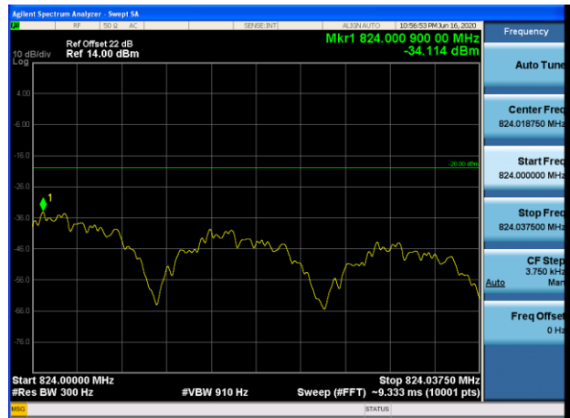
Channel 26789-1 tone offset 11, BW 15kHz, QPSK Frequency up to and including 37.5kHz
