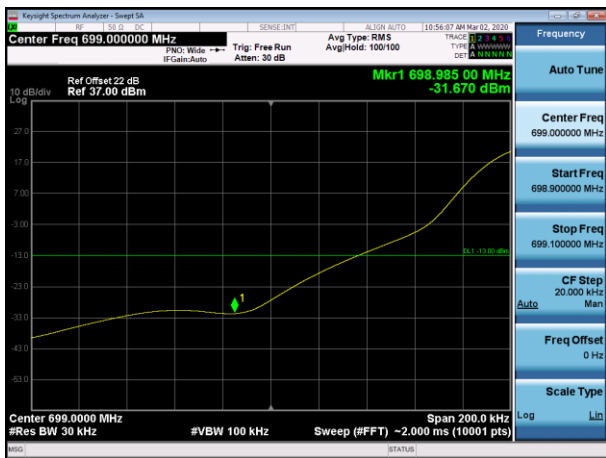
Channel 23012-1 tone offset 0, BW 3.75kHz, BPSK
