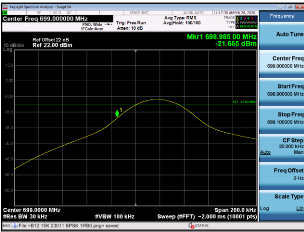
Channel 23011-1 tone offset 0, BW 15kHz, BPSK
