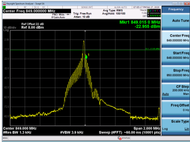
Channel 20649-1 tone offset 11, BW 15kHz, BPSK
