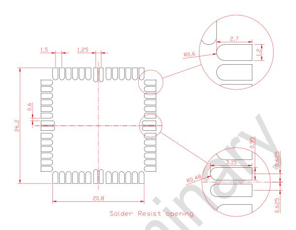
In order to easily rework the ML865C1 is suggested to consider on the application a 1.5 mm placement inhibit area around the module.
