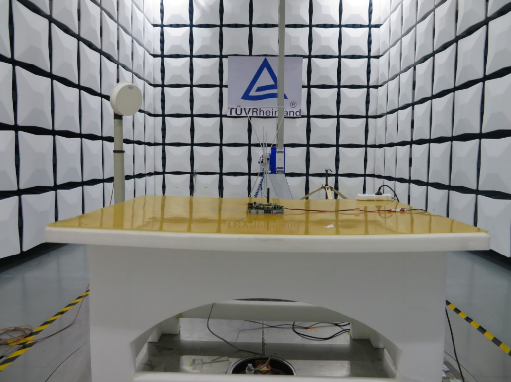
Photo 3: Radiated spurious emission for Above 1GHz
