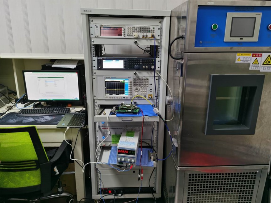
Photo 2: Radiated spurious emission for Below 1GHz
