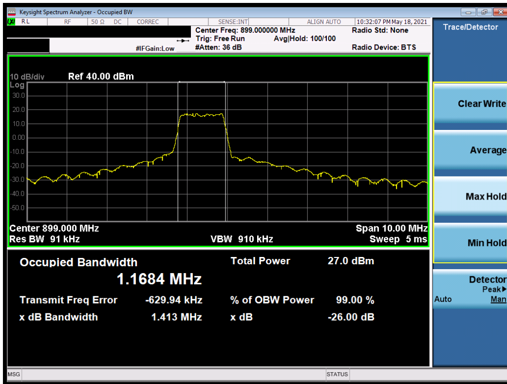
Plot 7-1. Occupied Bandwidth Plot (3MHz, QPSK, RB 6, RB Offset 0, NB=0)
