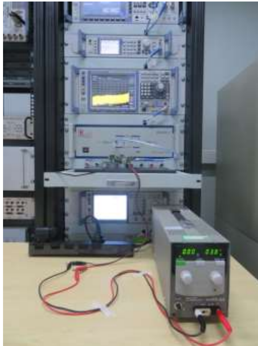
Photograph 1: Set-up for RF Output Power Measurement
