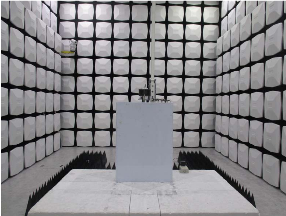
Description: Front View of Radiated Spurious Emission Test Setup (Horn)
