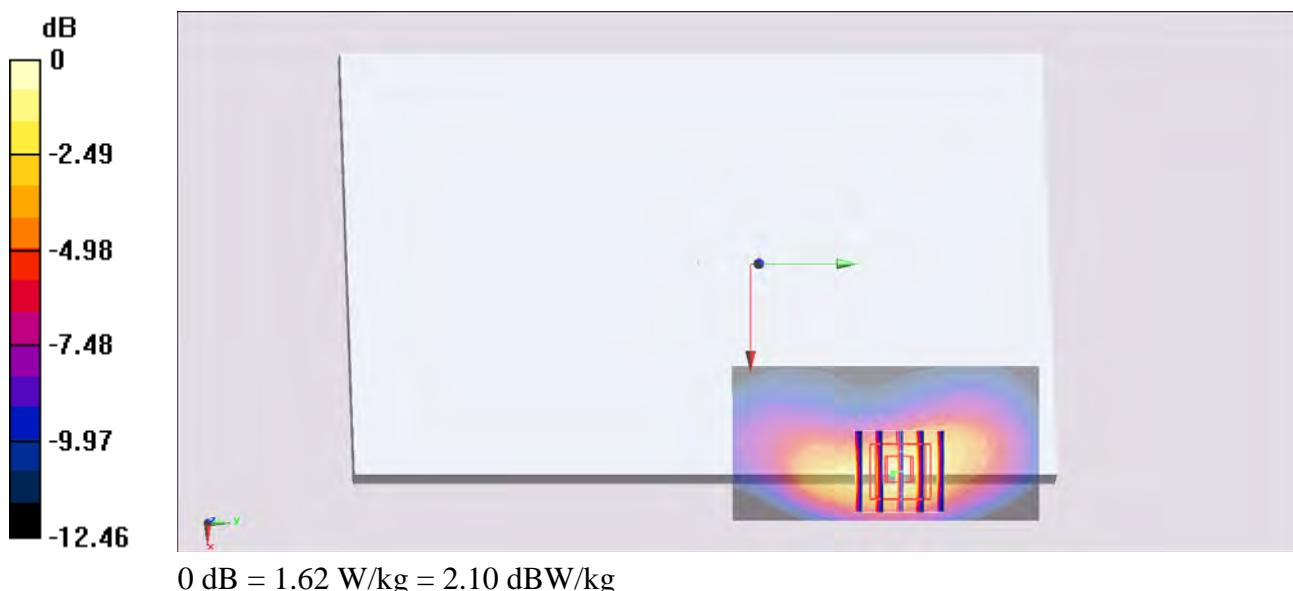
**#07\_LTE Band 13\_10M\_QPSK\_1RB\_0offset\_Curved surface of Edge1\_0cm\_Ch23230**
