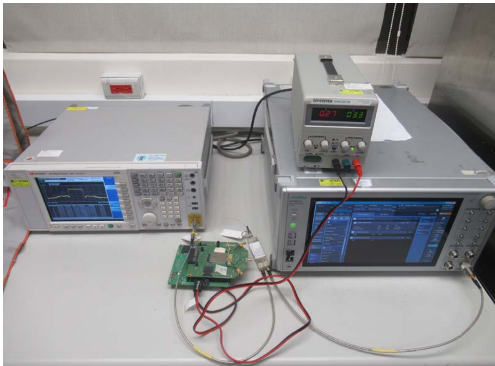
Conducted Setup Photo (Measurement at Antenna Port)
