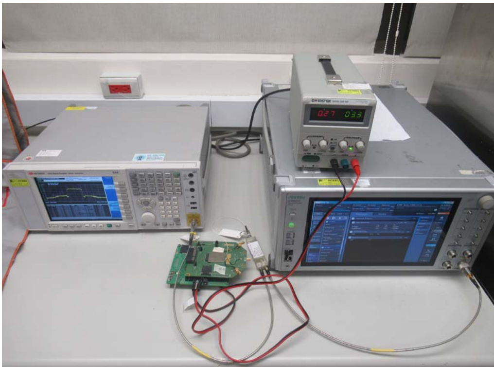
Conducted Setup Photo (Measurement at Antenna Port)
