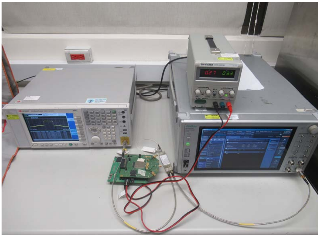
Conducted Setup Photo (Measurement at Antenna Port)
