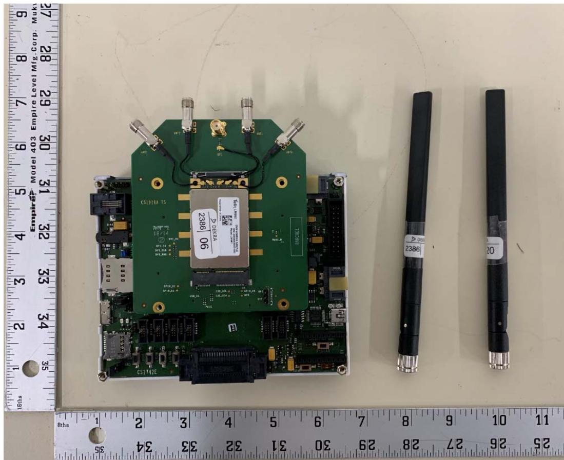
Evaluation board for LM960 & Antennas (Top side)
