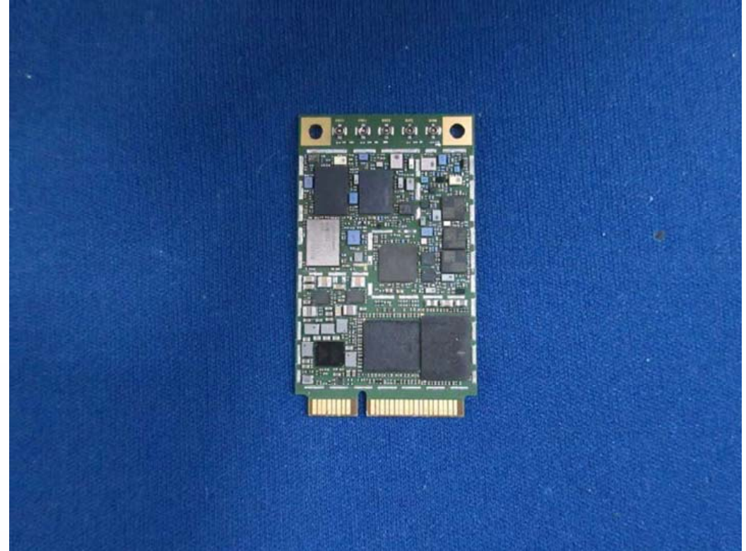
Internal photo of LM960 (Without Shield)
