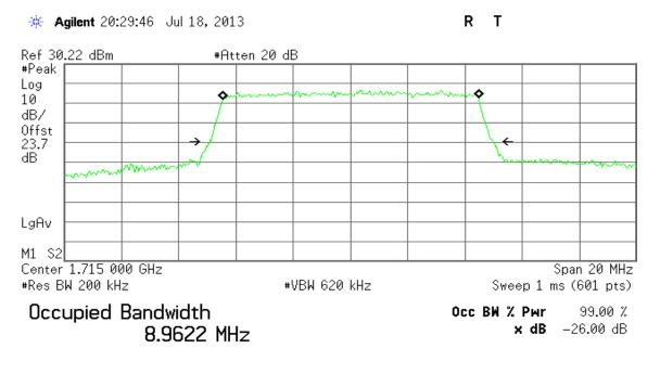
Transmit Freq Error 7.938 kHz x dB Bandwidth 9.911 MHz
