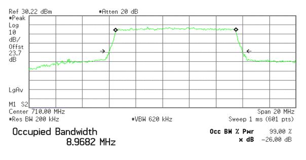
Transmit Freq Error 1.000 MHz x dB Bandwidth 9.915 MHz
