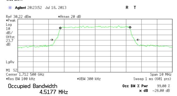
Transmit Freq Error 4.294 kHz x dB Bandwidth 5.091 MHz
