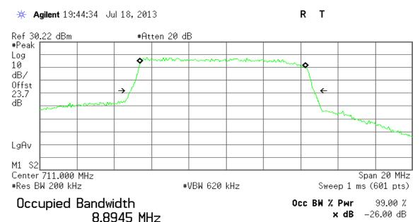
Transmit Freq Error -184.300 kHz x dB Bandwidth 9.846 MHz
