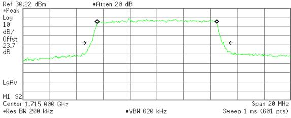
Occupied Bandwidth 8.9651 MHz Occ BW % Pwr 99.00 % x dB -26.00 dB
