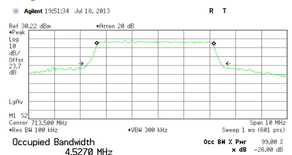
Transmit Freq Error -102.761 kHz x dB Bandwidth 5.170 MHz
