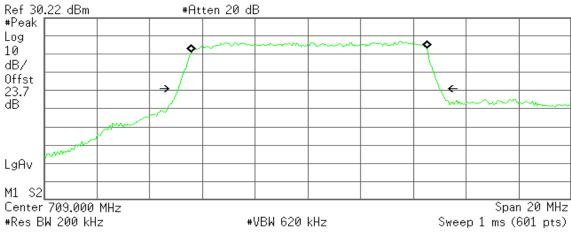
Occupied Bandwidth 8.9491 MHz Occ BW % Pwr 99.00 % x dB -26.00 dB
