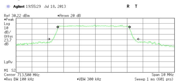
Occupied Bandwidth 4.5281 MHz Occ BW % Pwr 99.00 % **x dB** -26.00 dB
