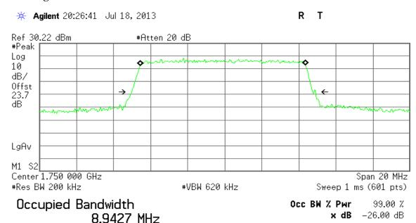
Transmit Freq Error -99.989 kHz x dB Bandwidth 9.931 MHz
