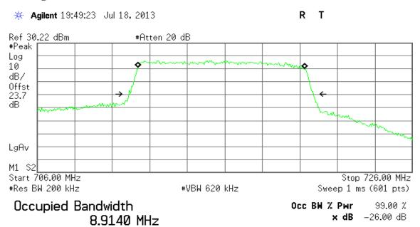
Transmit Freq Error -174.766 kHz x dB Bandwidth 9.846 MHz
