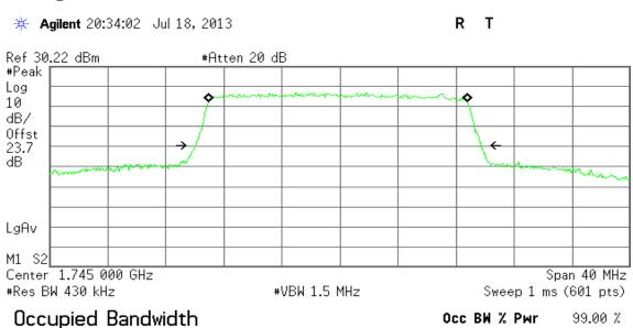
Transmit Freq Error -129.941 kHz x dB Bandwidth 19.676 MHz
