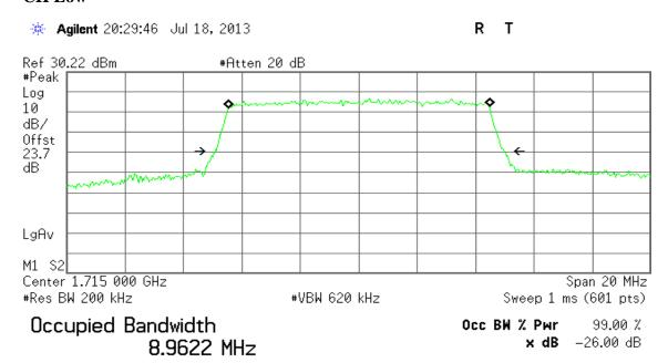
Transmit Freq Error 7.938 kHz x dB Bandwidth 9.911 MHz
