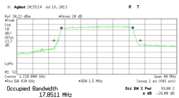
Transmit Freq Error 50.921 kHz x dB Bandwidth 19.684 MHz
