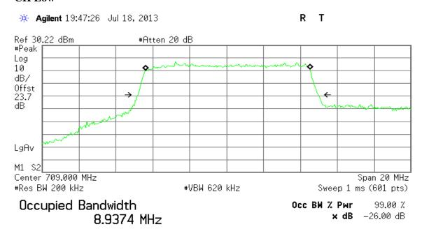
Transmit Freq Error 57.966 kHz x dB Bandwidth 9.795 MHz
