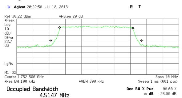
Transmit Freq Error -88.153 kHz x dB Bandwidth 5.093 MHz
