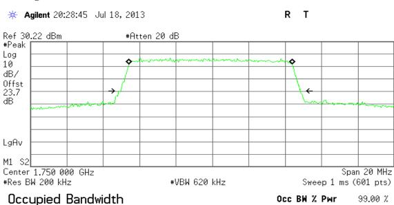
Transmit Freq Error -97.183 kHz x dB Bandwidth 9.882 MHz
