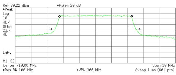
Occupied Bandwidth 4.5160 MHz Occ BW % Pwr 99.00 % **x dB** -26.00 dB
