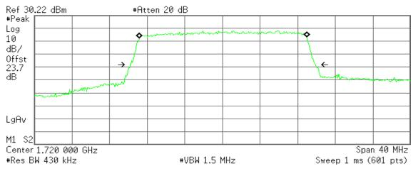
Occupied Bandwidth 17.8180 MHz Occ BW % Pwr 99.00 % x dB -26.00 dB
