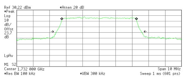
Occupied Bandwidth 4.5266 MHz Occ BW % Pwr 99.00 % **x dB** -26.00 dB
