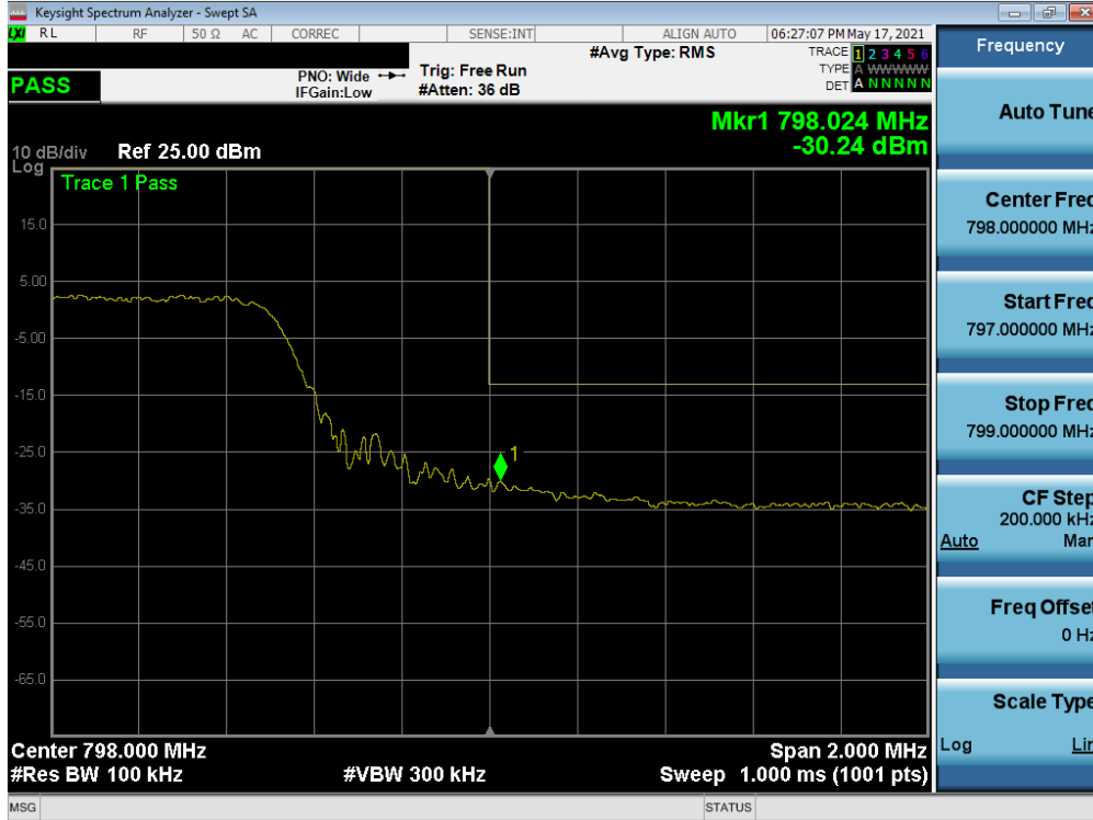
Plot 7-10. Upper Band Edge Plot (LTE Band 14, 10MHz QPSK - RB Size 50)
