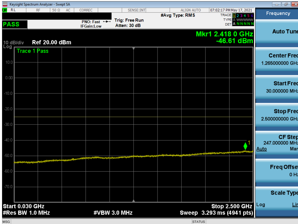
Plot 7-12. Conducted Spurious Plot (LTE Band 7 - 20MHz QPSK - RB Size 1, RB Offset 0 - Mid Channel)
