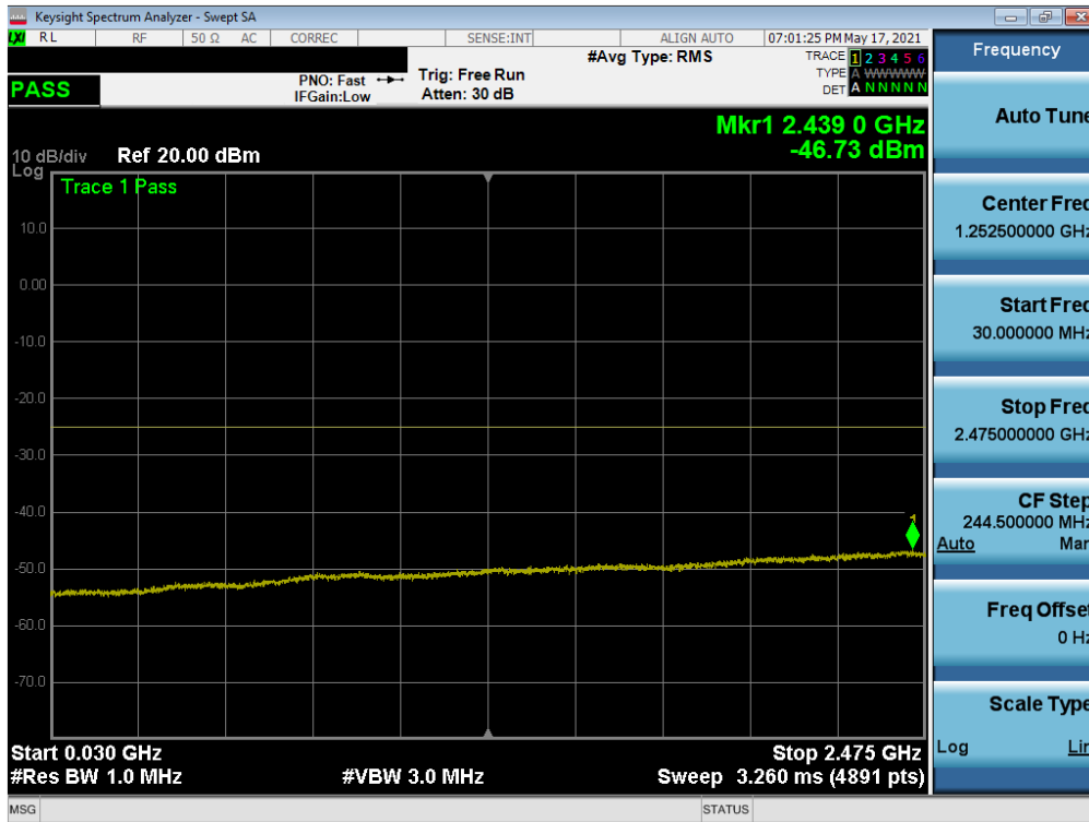
Plot 7-9. Conducted Spurious Plot (LTE Band 7 - 20MHz QPSK - RB Size 1, RB Offset 0 - Low Channel)
