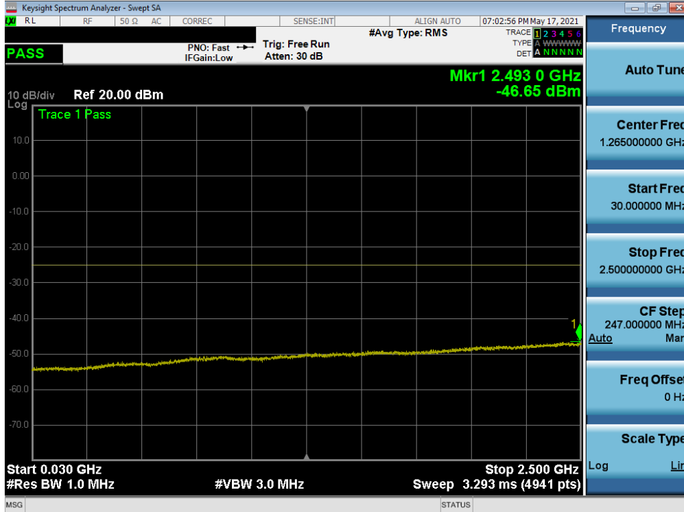
Plot 7-15. Conducted Spurious Plot (LTE Band 7 - 20MHz QPSK - RB Size 1, RB Offset 0 - High Channel)
