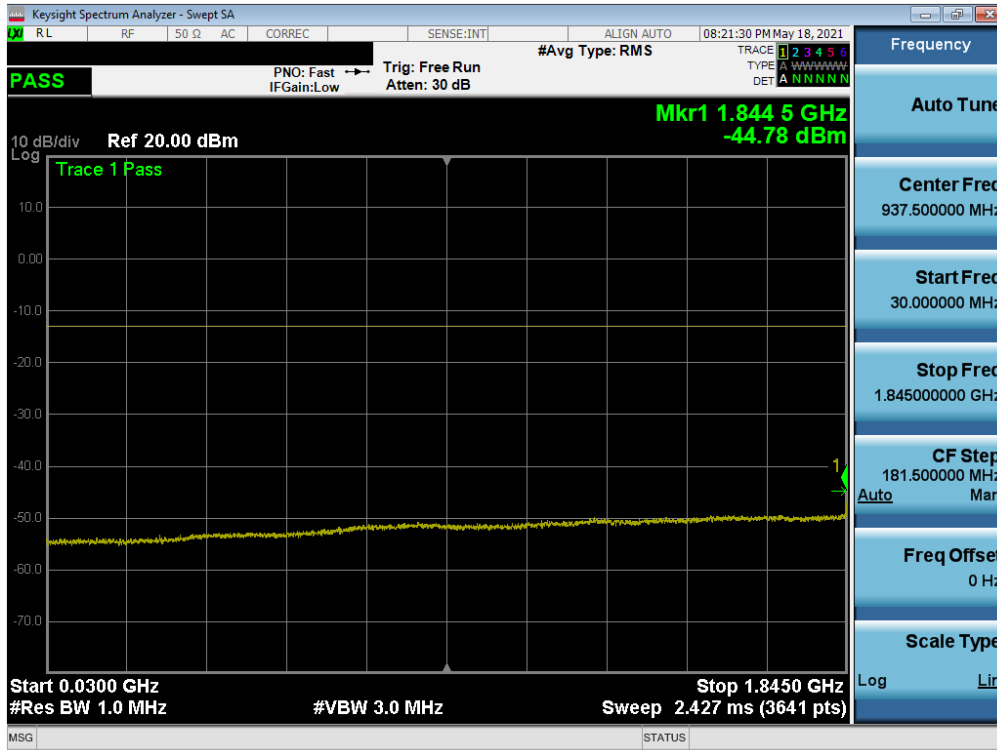
Plot 7-34. Conducted Spurious Plot (WCDMA Ch. 9262)
