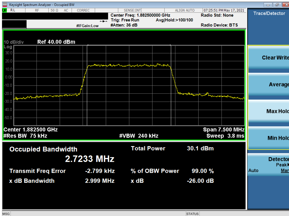
Plot 7-10. Occupied Bandwidth Plot (LTE Band 25/2 - 3MHz 16-QAM - Full RB)
