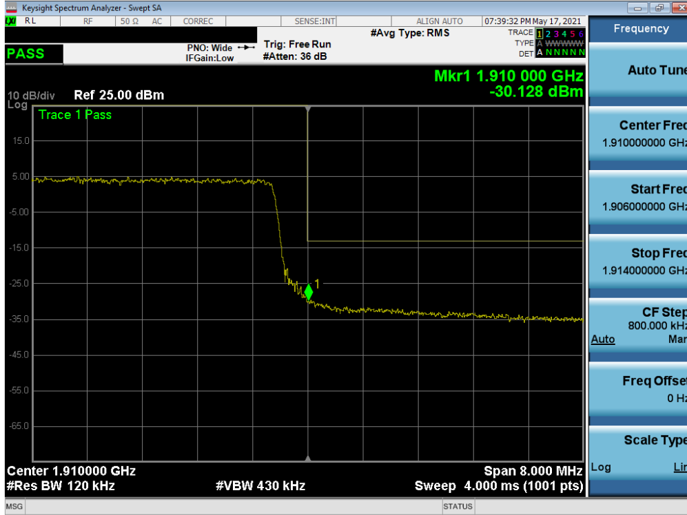
Plot 7-57. Upper Band Edge Plot (LTE Band 2 - 10MHz QPSK – Full RB)
