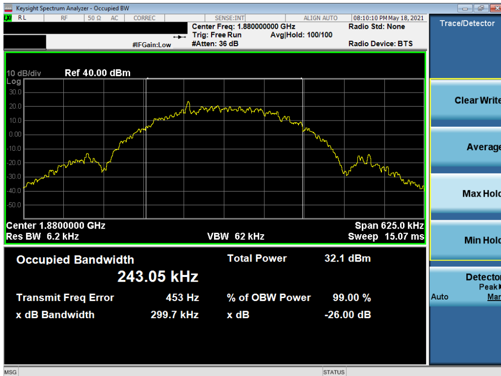
Plot 7-14. Occupied Bandwidth Plot (EDGE, Ch. 661)
