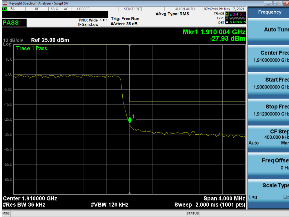
Plot 7-69. Upper Band Edge Plot (LTE Band 2 - 3MHz QPSK – Full RB)
