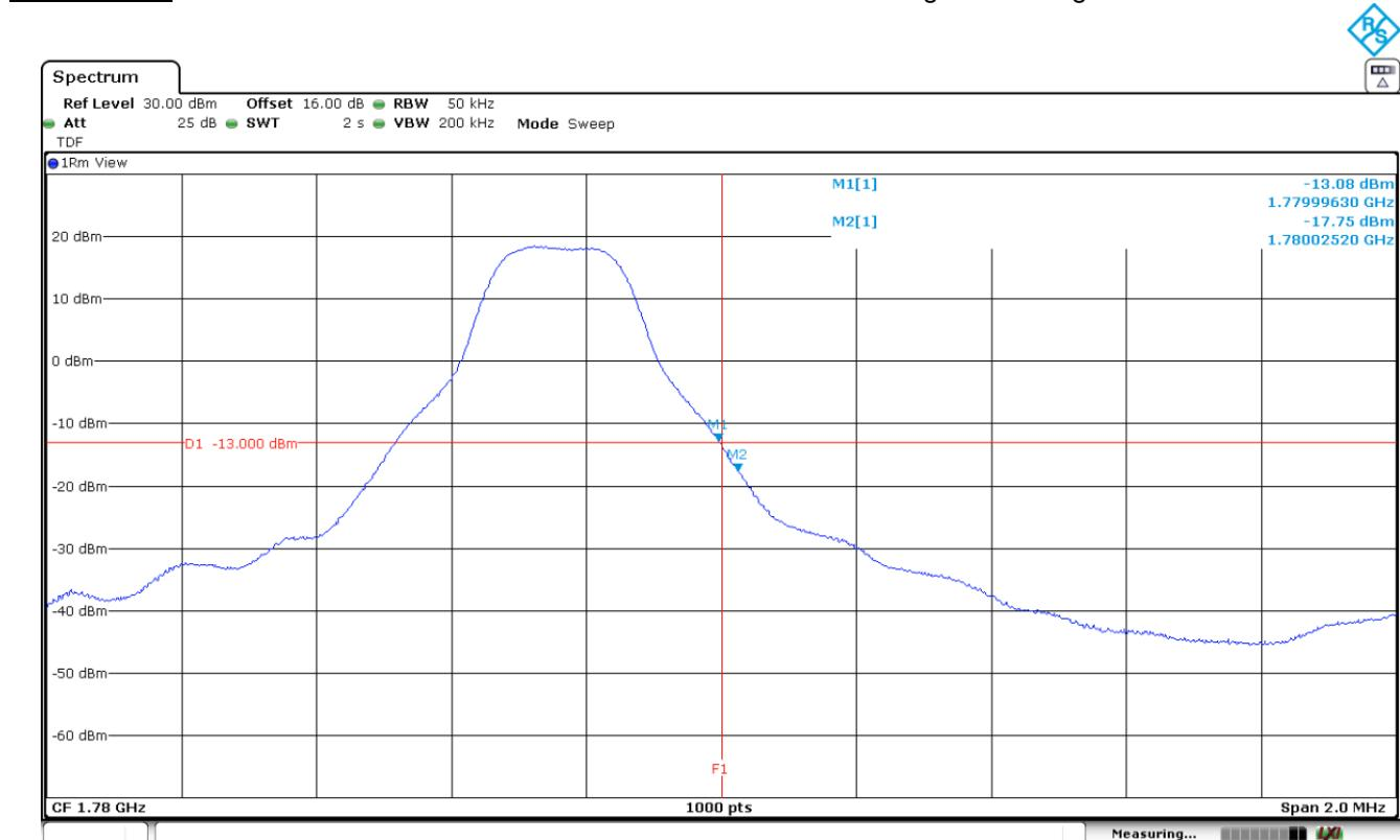
LTE Band 66. QPSK MODULATION. BW=3 MHz. RB=All. Offset=0. Low and High Block Edges:
