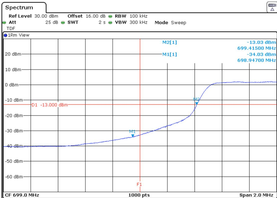
LTE Band 12. QPSK MODULATION. BW=10 MHz. RB=All. Offset=0. High Block Edges:
