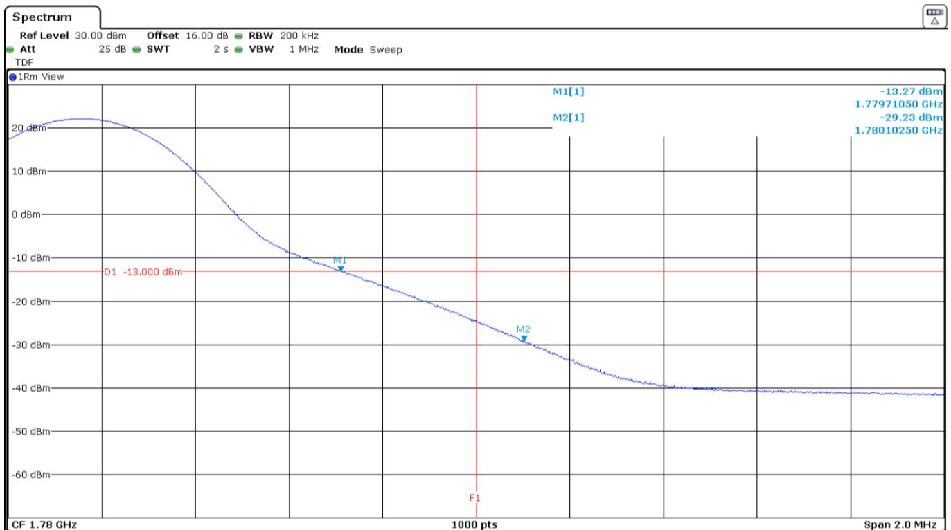
LTE Band 66. QPSK MODULATION. BW=15 MHz. RB=All. Offset=0. Low and High Block Edges:
