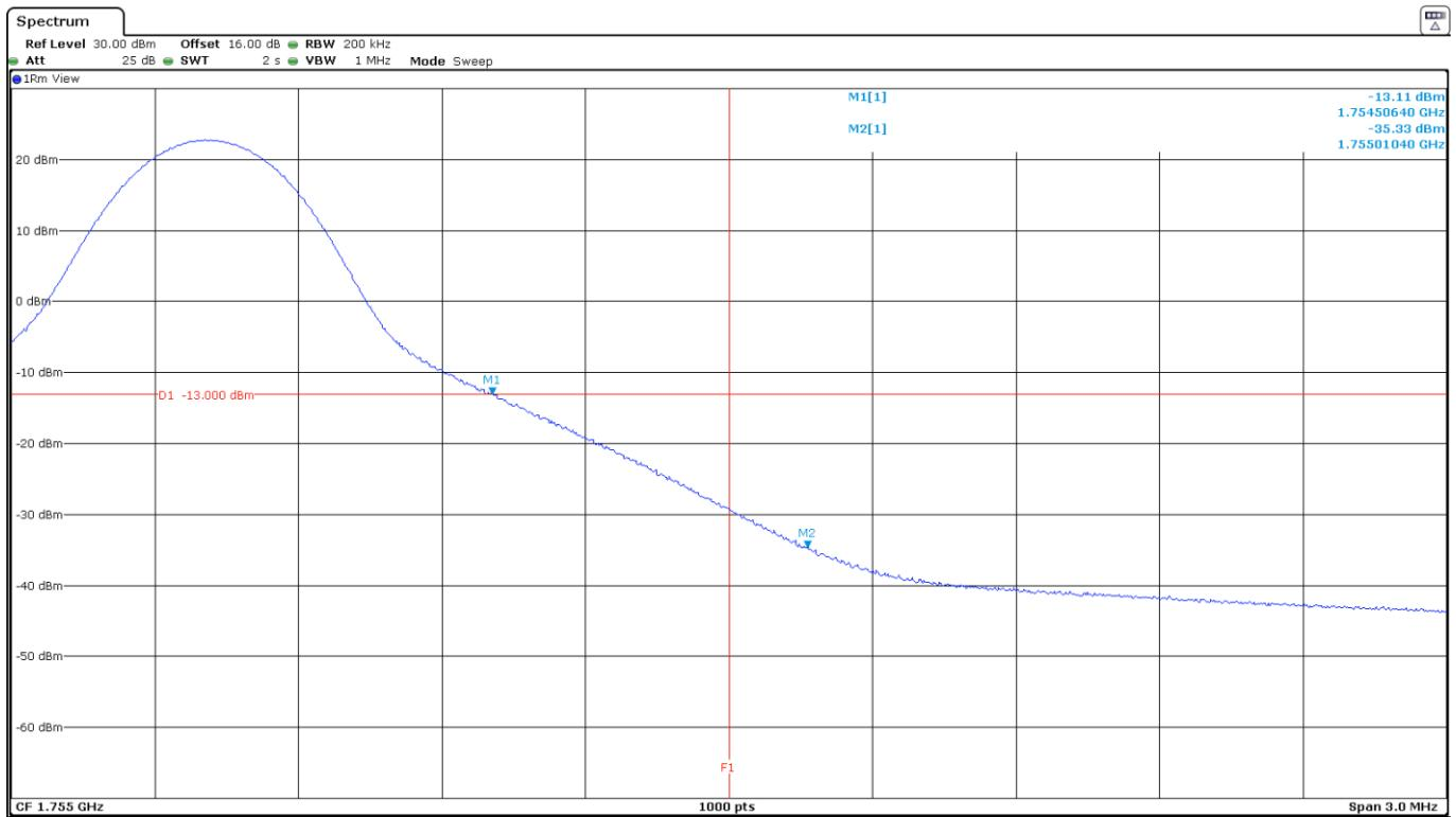
LTE Band 4. QPSK MODULATION. BW=20 MHz. RB>All. Offset=0. High Block Edge:
