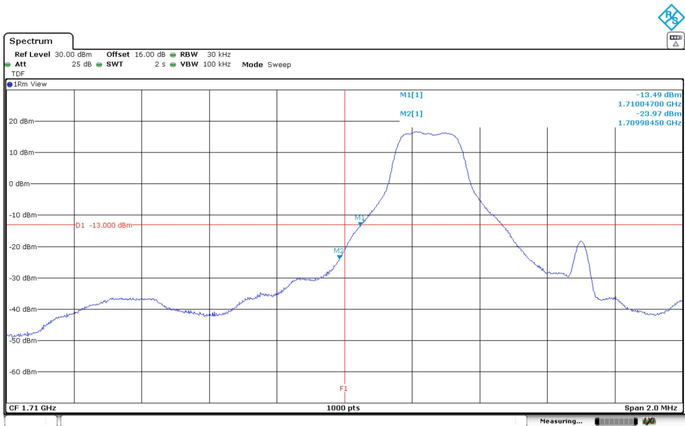
LTE Band 66. QPSK MODULATION. BW=1.4 MHz. RB=1. Offset=Max. High Block Edge:
