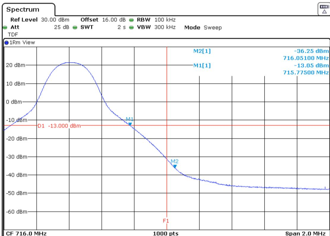
LTE Band 12. QPSK MODULATION. BW=10 MHz. RB=All. Offset=0. Low Block Edges:
