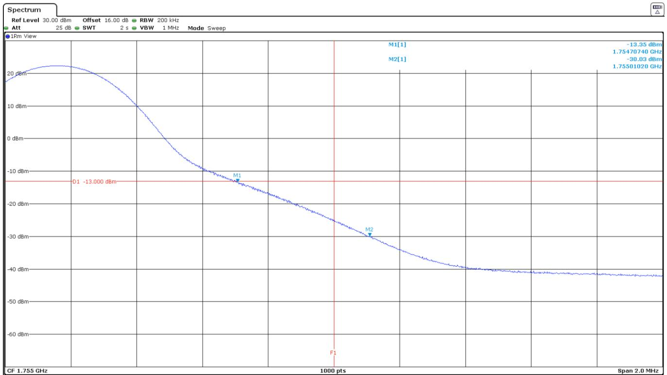
LTE Band 4. QPSK MODULATION. BW=15 MHz. RB>All. Offset=0. High Block Edge:
