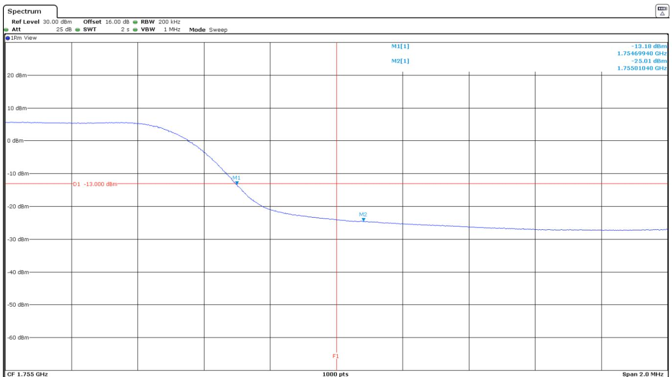
LTE Band 4. QPSK MODULATION. BW=15 MHz. RB=1. Offset=Max. High Block Edge:
