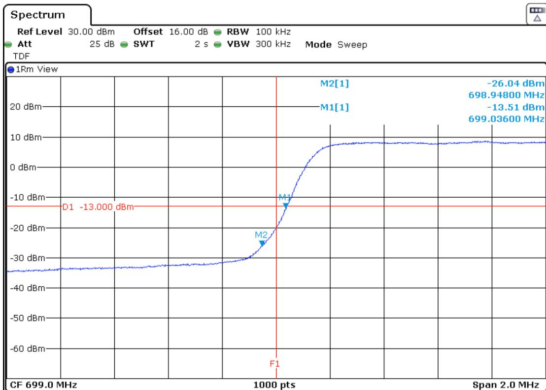
LTE Band 12. QPSK MODULATION. BW=3 MHz. RB=All. Offset=0. High Block Edges:
