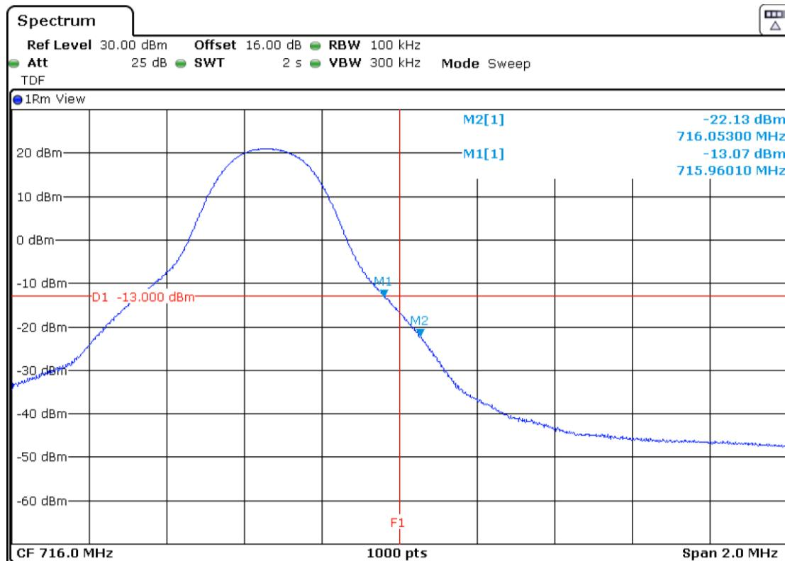
LTE Band 12. QPSK MODULATION. BW=5 MHz. RB=All. Offset=0. Low Block Edges:
