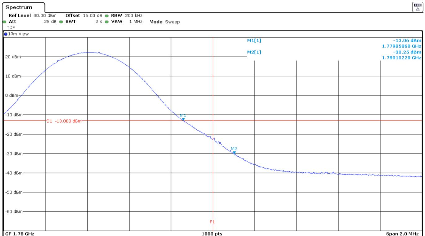
LTE Band 66. QPSK MODULATION. BW=10 MHz. RB=All. Offset=0. Low and High Block Edges:
