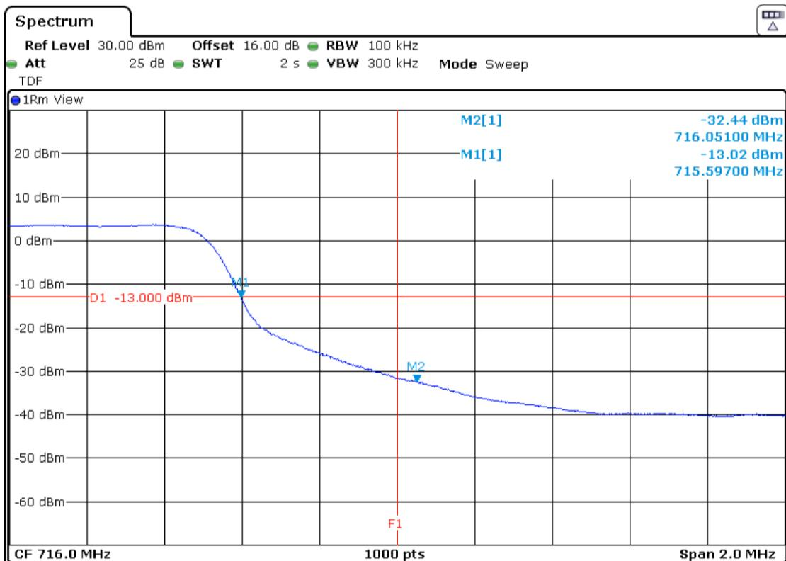
LTE Band 66. QPSK MODULATION. BW=1.4 MHz. RB=1. Offset=0. Low Block Edge:
