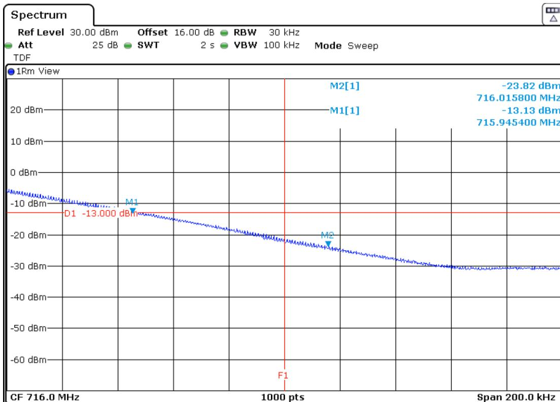
LTE Band 12. QPSK MODULATION. BW=1.4 MHz. RB=All. Offset=0. Low and High Block Edges:
