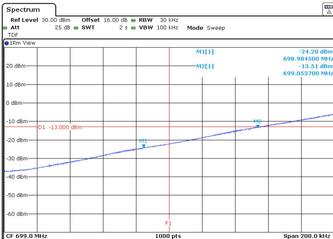
LTE Band 12. QPSK MODULATION. BW=1.4 MHz. RB=1. Offset=Max. High Block Edge:
