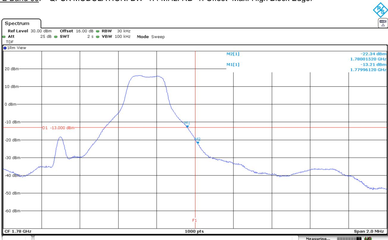
LTE Band 66. QPSK MODULATION. BW=1.4 MHz. RB=All. Offset=0. Low and High Block Edges:
