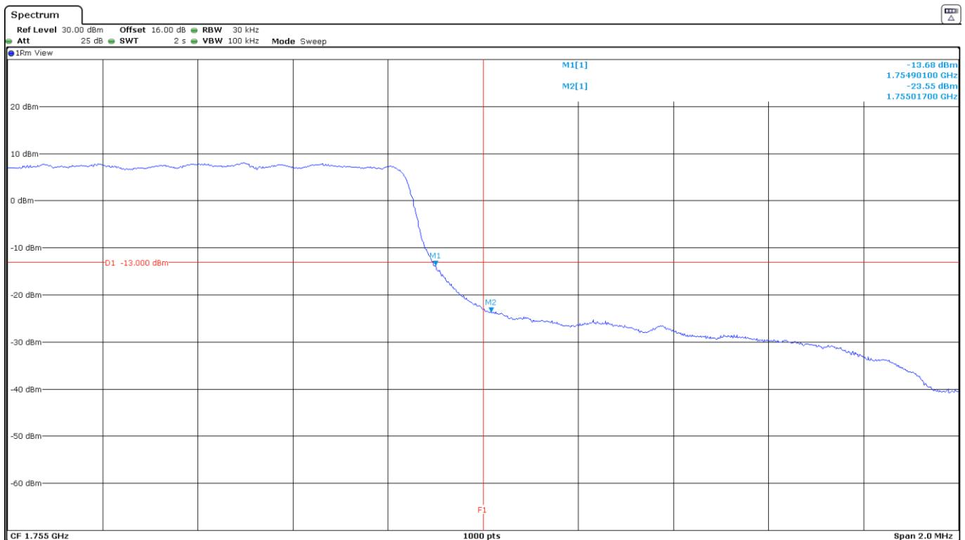
LTE Band 4. QPSK MODULATION. BW=3 MHz. RB=1. Offset=Max. High Block Edge:
