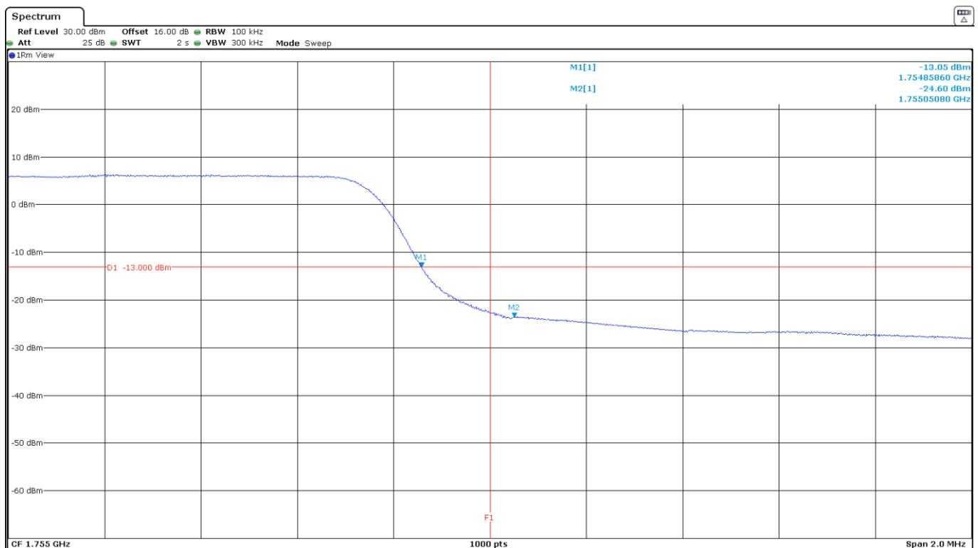
LTE Band 4. QPSK MODULATION. BW=10 MHz. RB=1. Offset=Max. High Block Edge:
