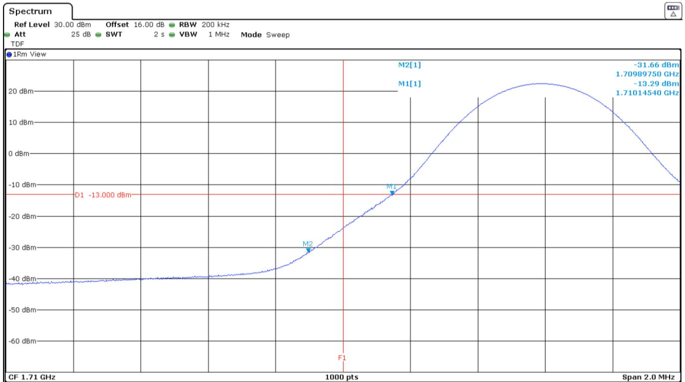
LTE Band 66. QPSK MODULATION. BW=10 MHz. RB=1. Offset=Max. High Block Edge:
