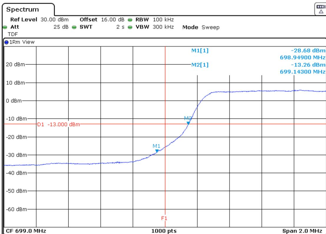
LTE Band 12. QPSK MODULATION. BW=5 MHz. RB=All. Offset=0. High Block Edges:
