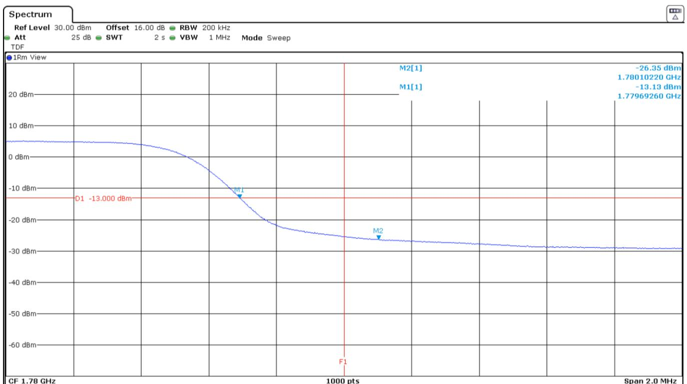
LTE Band 66. QPSK MODULATION. BW=15 MHz. RB=1. Offset=0. Low Block Edge:
