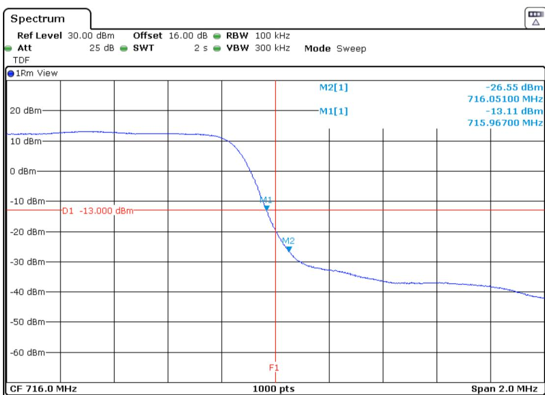
LTE Band 12. QPSK MODULATION. BW=3 MHz. RB=1. Offset=0. Low Block Edge:
