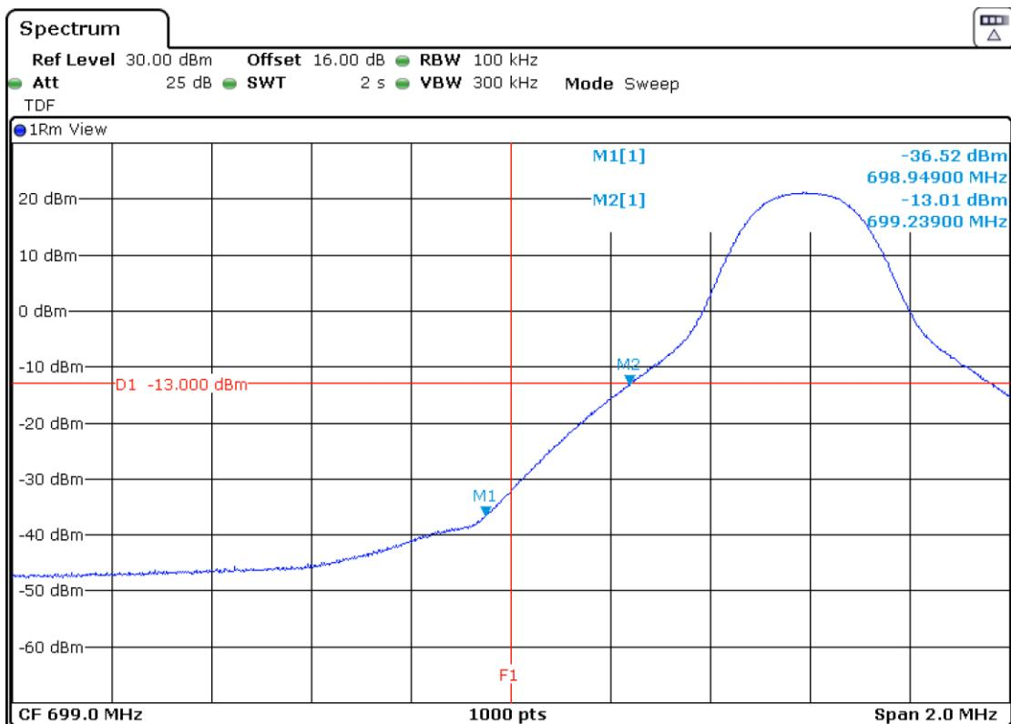
LTE Band 12. QPSK MODULATION. BW=10 MHz. RB=1. Offset=Max. High Block Edge:
