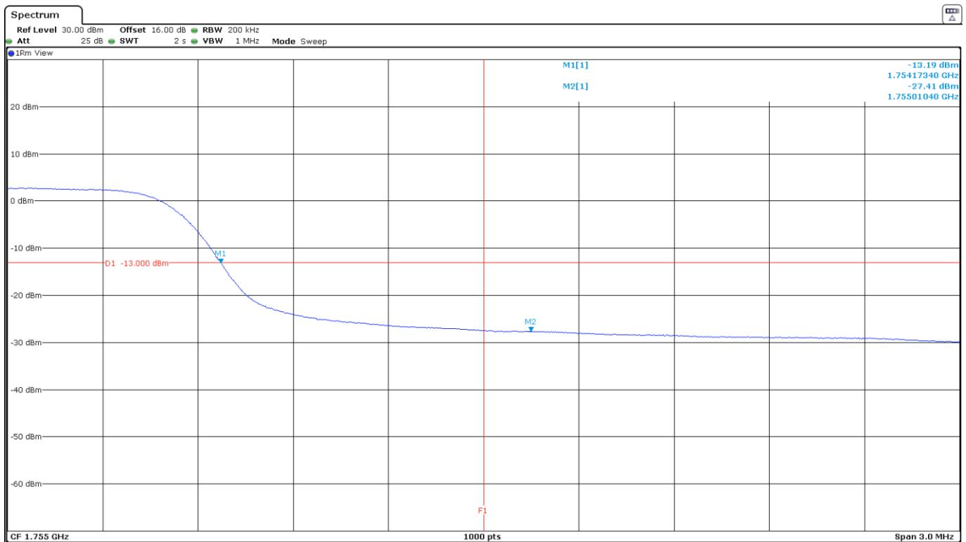
LTE Band 12. QPSK MODULATION. BW=1.4 MHz. RB=1. Offset=0. Low Block Edge:
