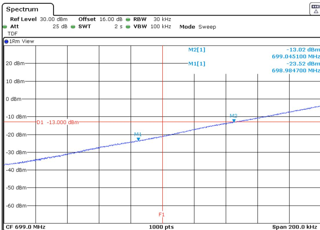
LTE Band 12. QPSK MODULATION. BW=3 MHz. RB=1. Offset=Max. High Block Edge:
