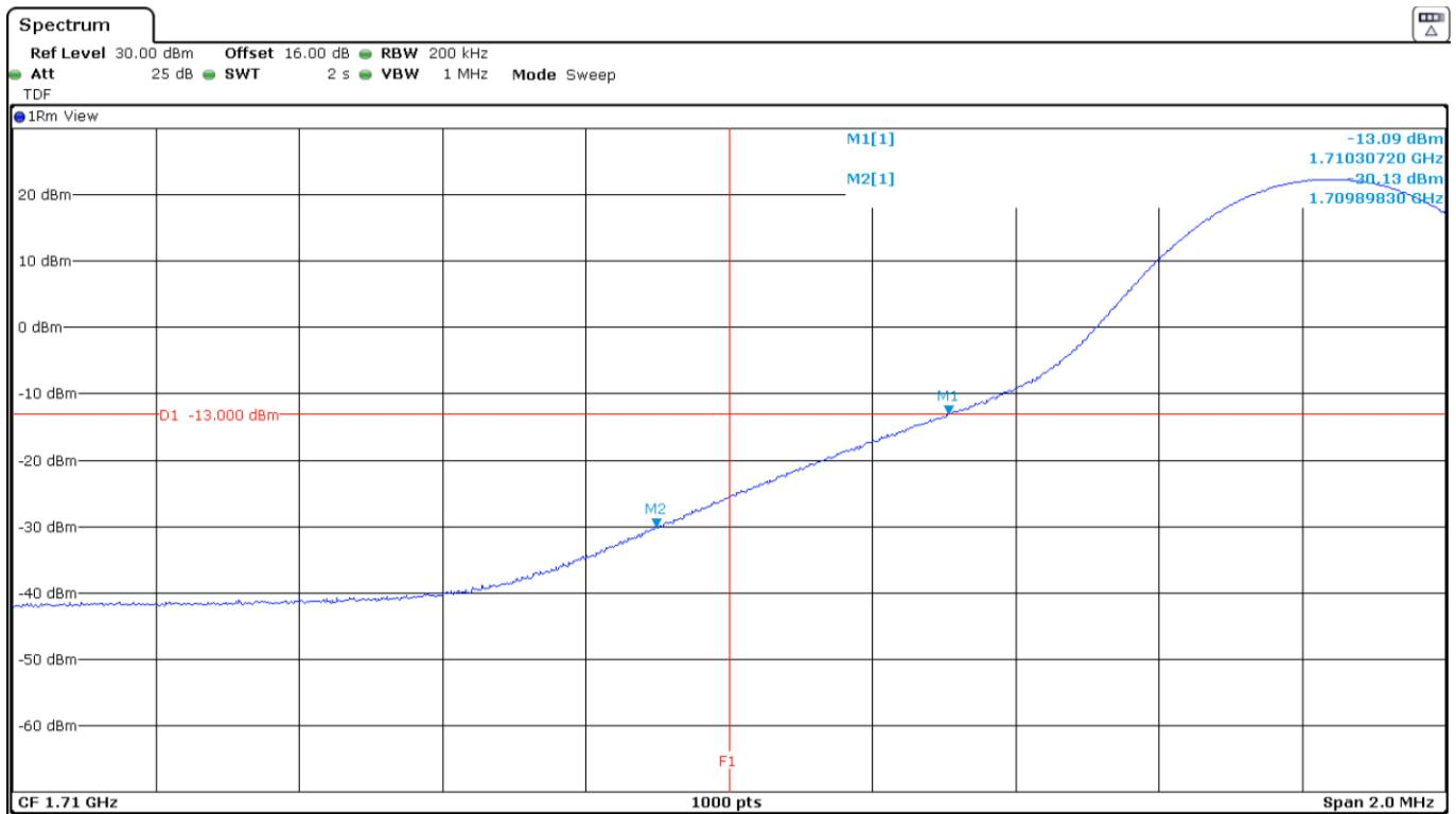
LTE Band 66. QPSK MODULATION. BW=15 MHz. RB=1. Offset=Max. High Block Edge:
