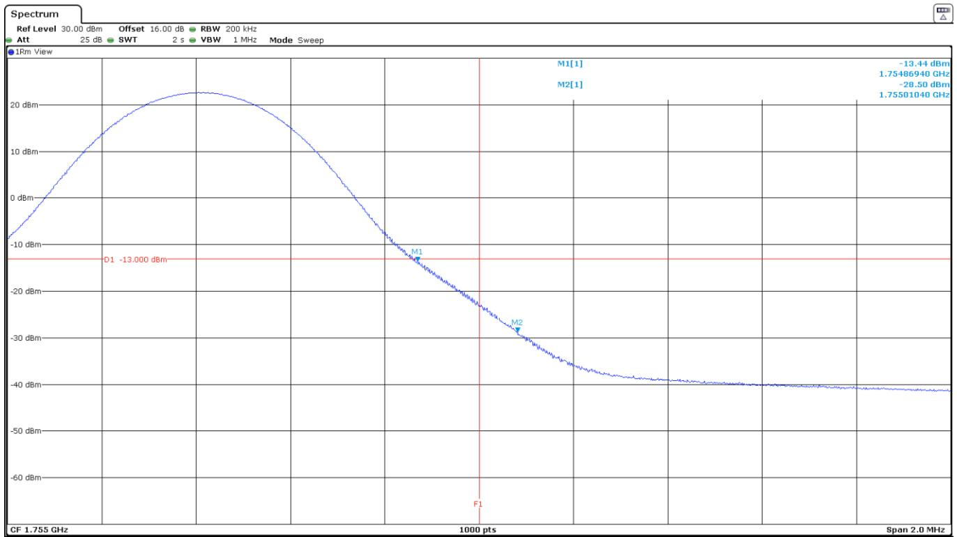
LTE Band 4. QPSK MODULATION. BW=10 MHz. RB=All. Offset=0. High Block Edge:
