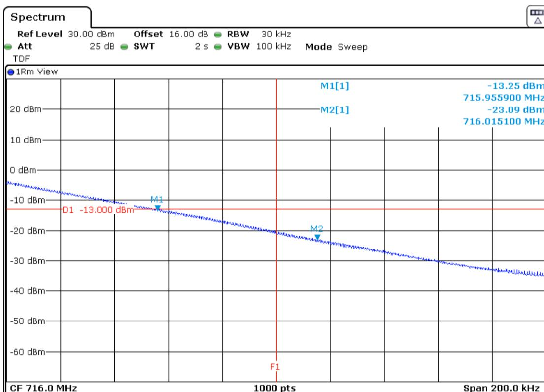
LTE Band 12. QPSK MODULATION. BW=3 MHz. RB=All. Offset=0. Low Block Edges:
