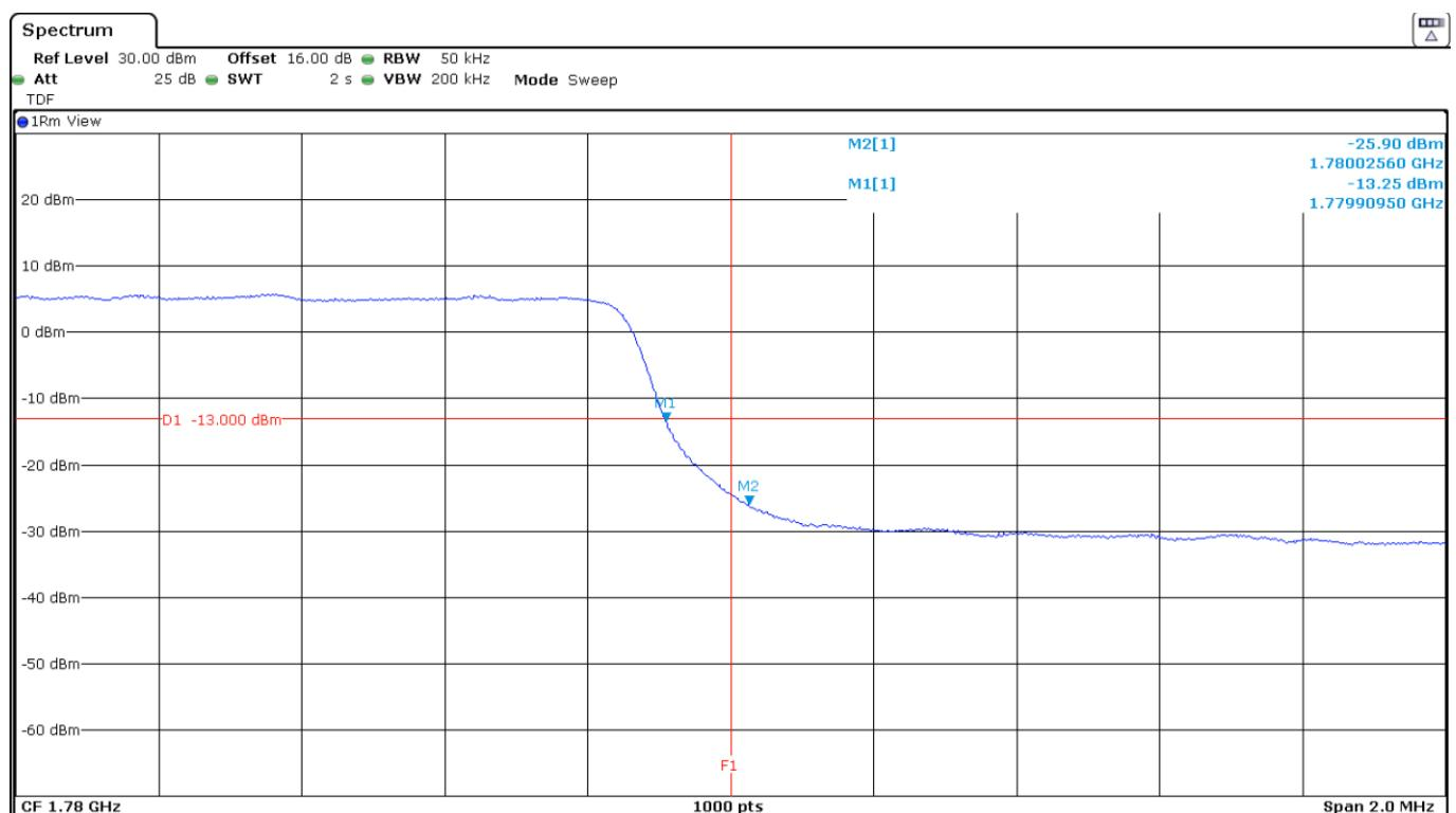
LTE Band 66. QPSK MODULATION. BW=5 MHz. RB=1. Offset=0. Low Block Edge:
