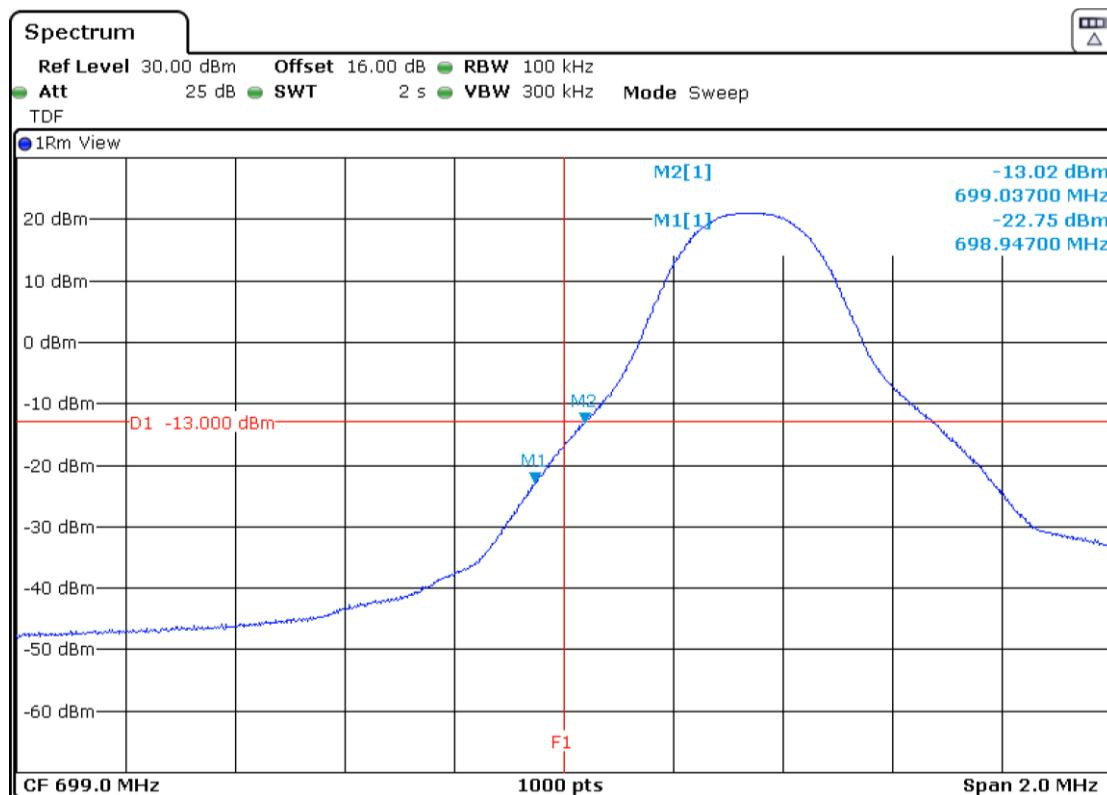
LTE Band 12. QPSK MODULATION. BW=5 MHz. RB=1. Offset=Max. High Block Edge:
