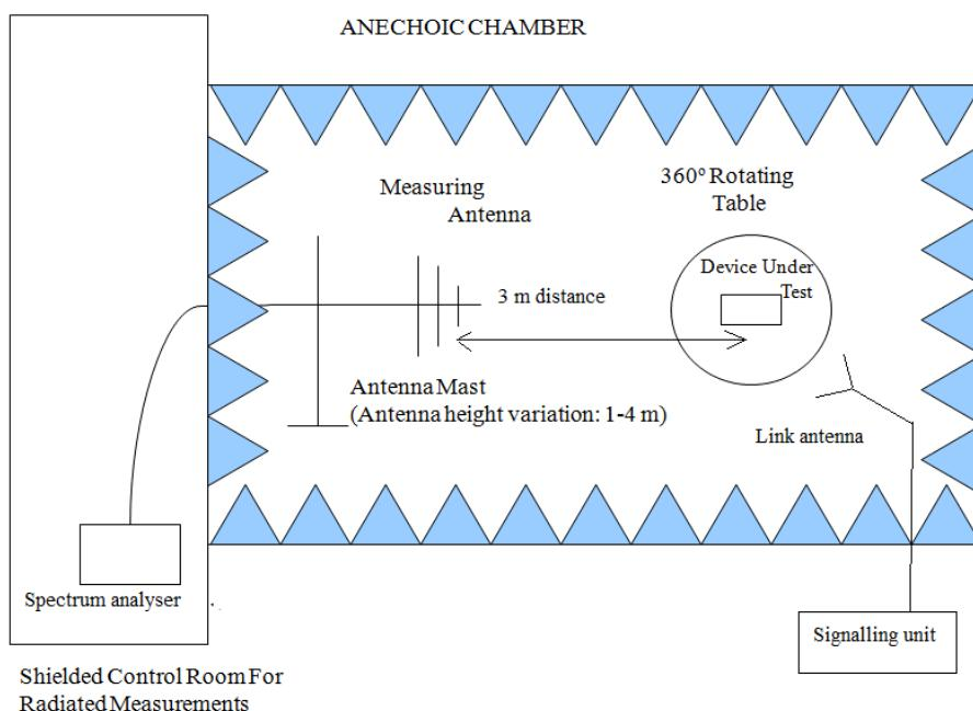
Radiated measurements above 1 GHz.
