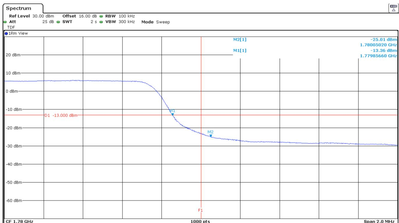
LTE Band 66. QPSK MODULATION. BW=10 MHz. RB=1. Offset=0. Low Block Edge:
