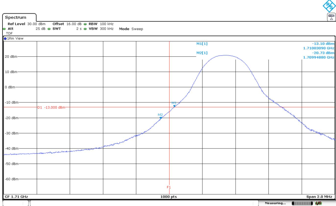
LTE Band 66. QPSK MODULATION. BW=5 MHz. RB=1. Offset=Max. High Block Edge:
