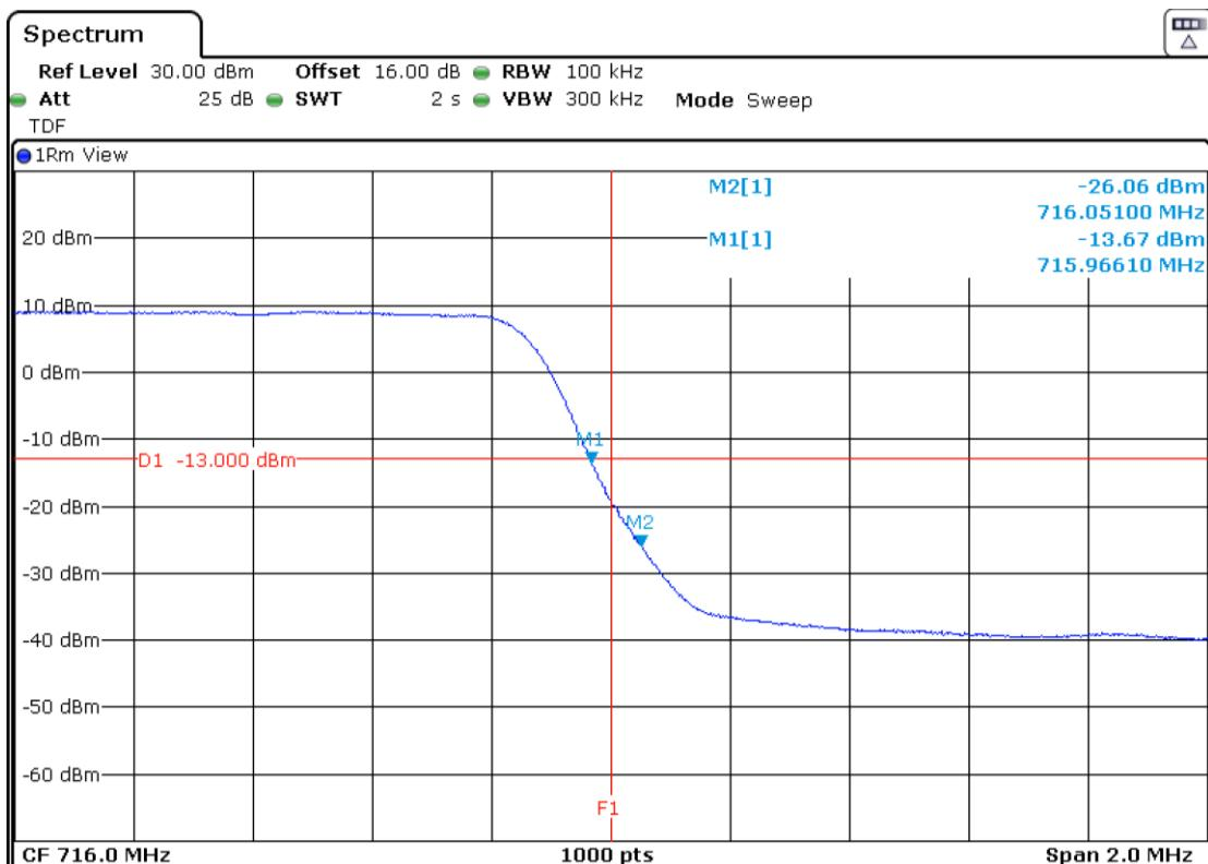
LTE Band 12. QPSK MODULATION. BW=5 MHz. RB=1. Offset=0. Low Block Edge:
