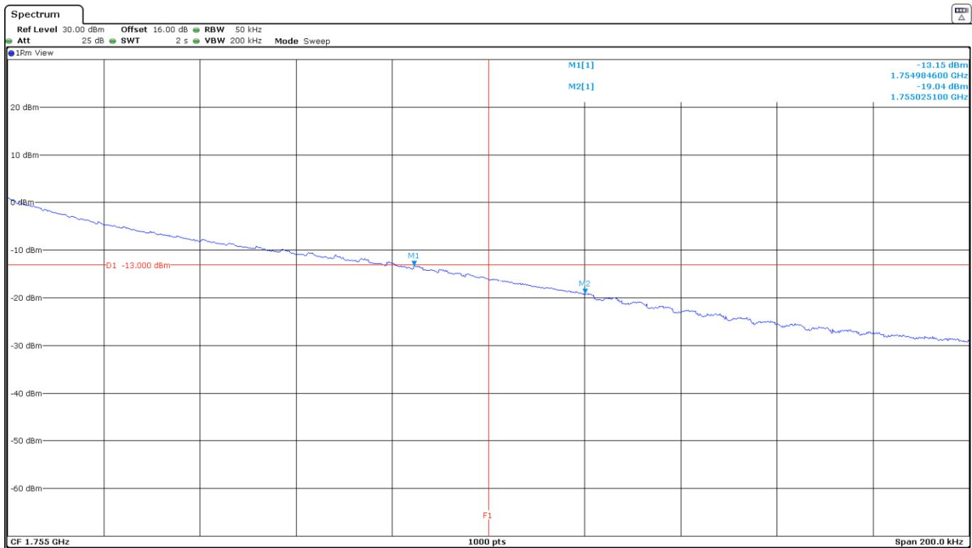
LTE Band 4. QPSK MODULATION. BW=3 MHz. RB=All. Offset=0. High Block Edge:
