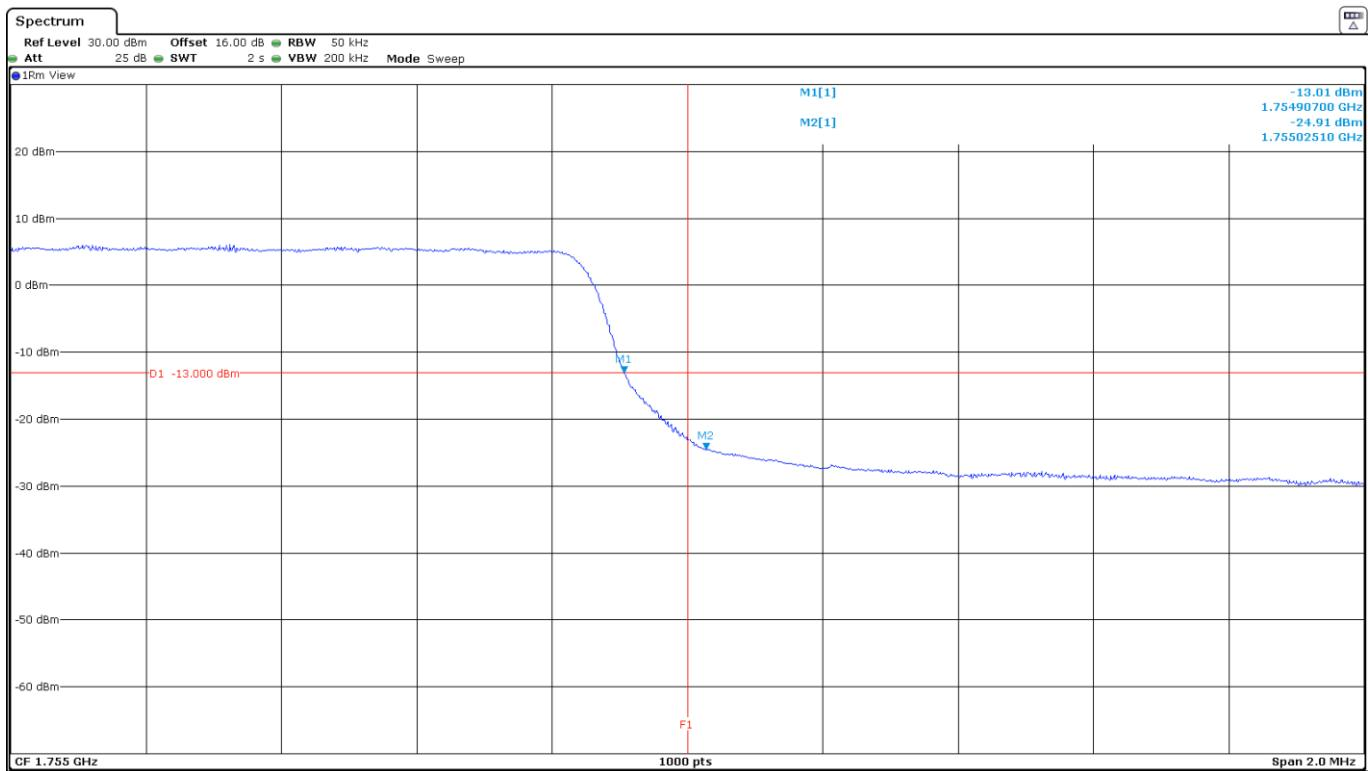
LTE Band 4. QPSK MODULATION. BW=5 MHz. RB=1. Offset=Max. High Block Edge:
