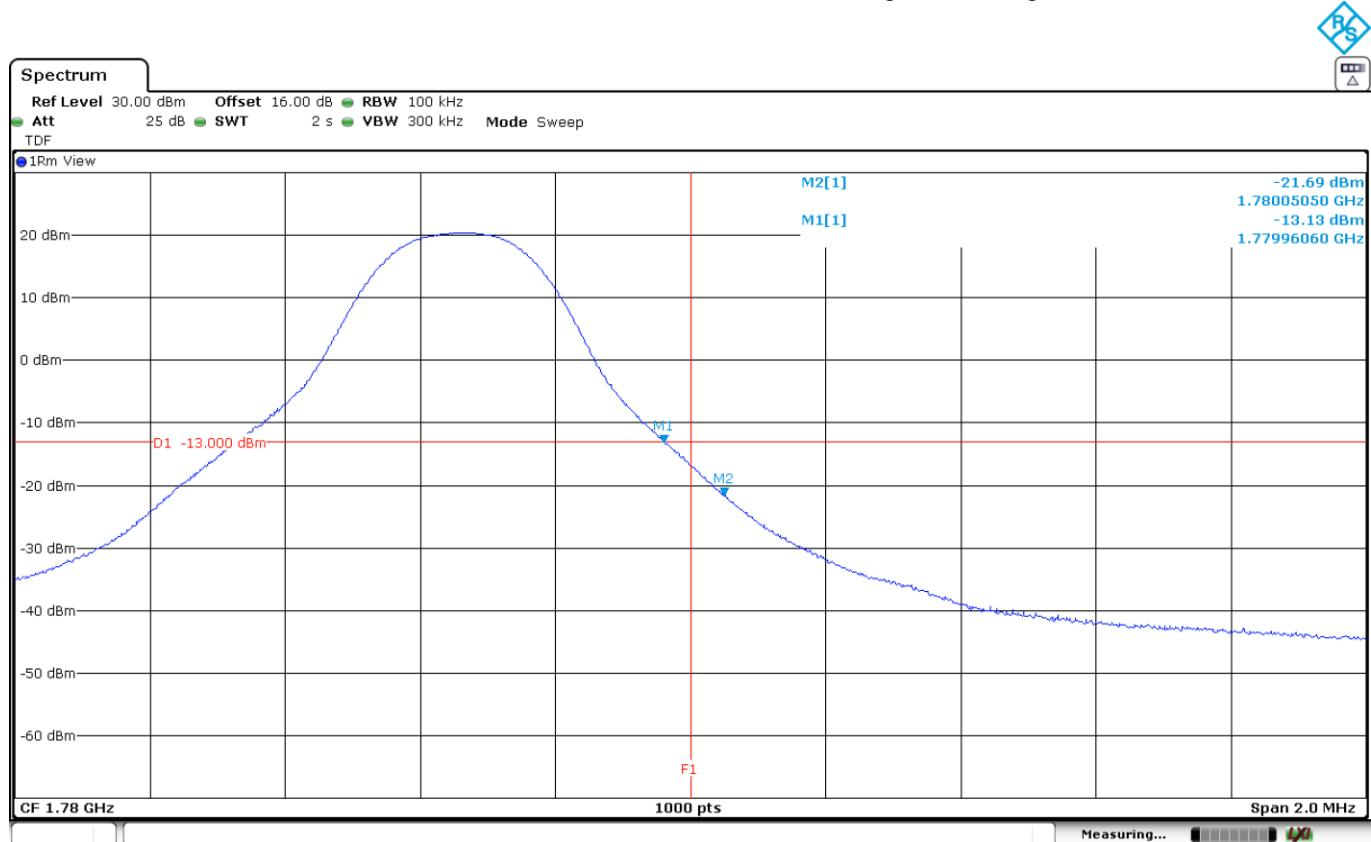
LTE Band 66. QPSK MODULATION. BW=5 MHz. RB=All. Offset=0. Low and High Block Edges:
