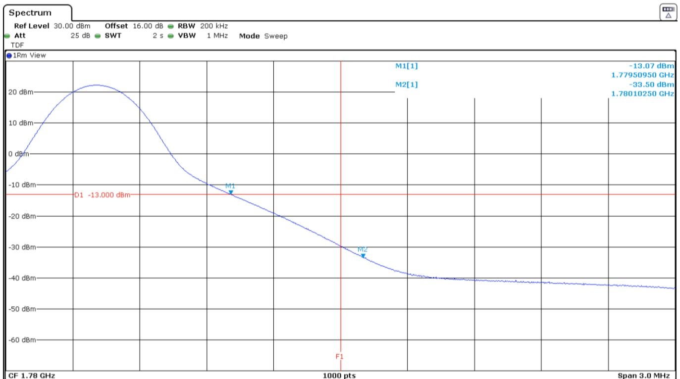
LTE Band 66. QPSK MODULATION. BW=20 MHz. RB=All. Offset=0. Low and High Block Edges:
