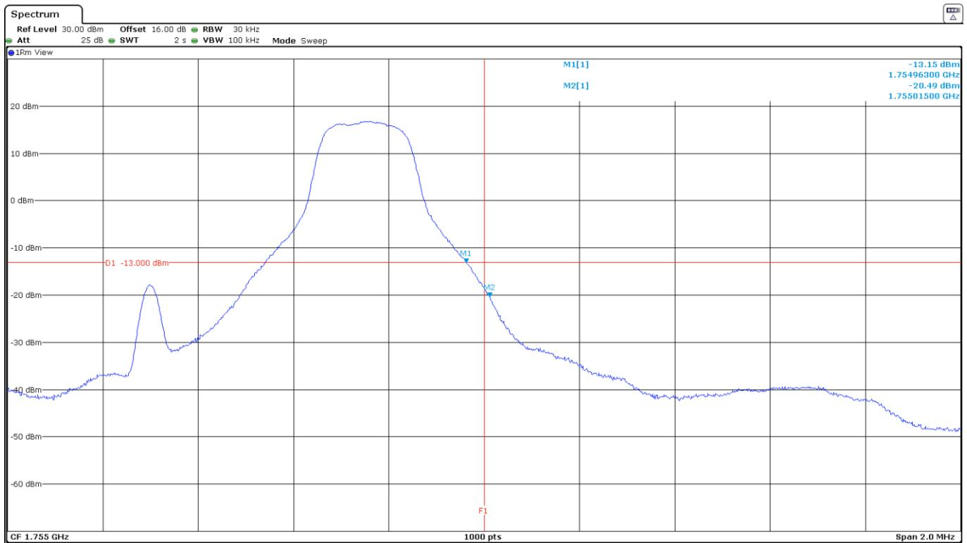
LTE Band 4. QPSK MODULATION. BW=1.4 MHz. RB=All. Offset=0. High Block Edge:
