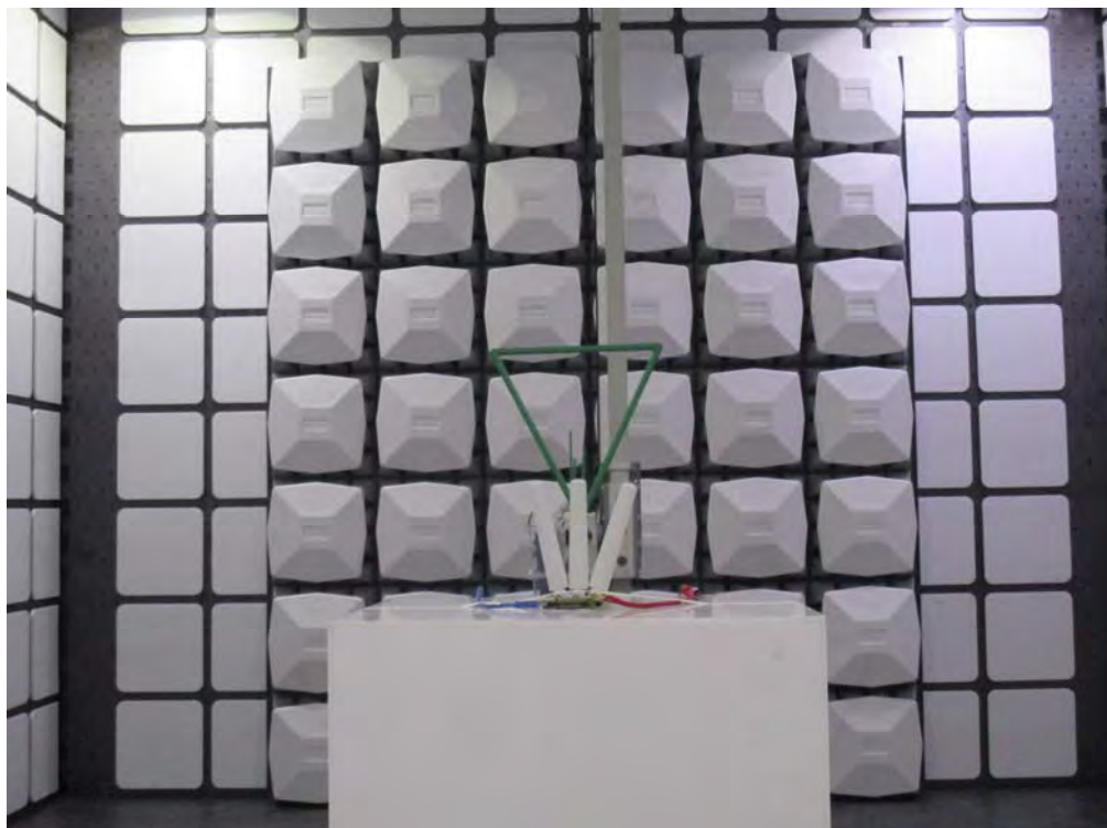
Description: Back View of Radiated Spurious Emission Test Setup
