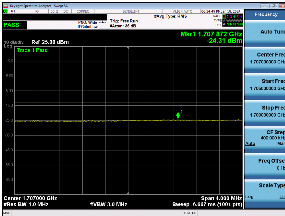
Plot 7-69. Lower Extended Band Edge Plot (LTE Band 66/4 - 15MHz QPSK – Full RB)
