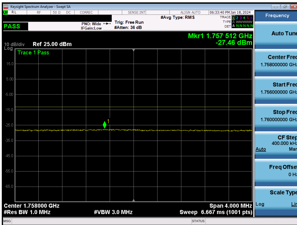
Plot 7-65. Upper Extended Band Edge Plot (LTE Band 4 - 20MHz QPSK – Full RB)
