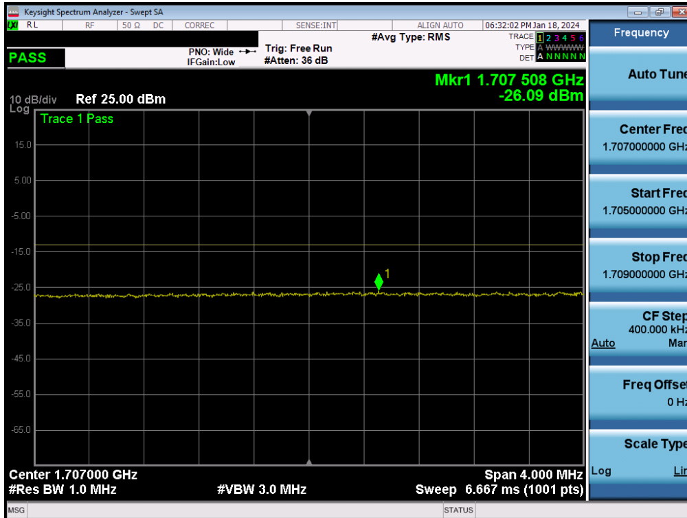
Plot 7-63. Lower Extended Band Edge Plot (LTE Band 66/4 - 20MHz QPSK – Full RB)
