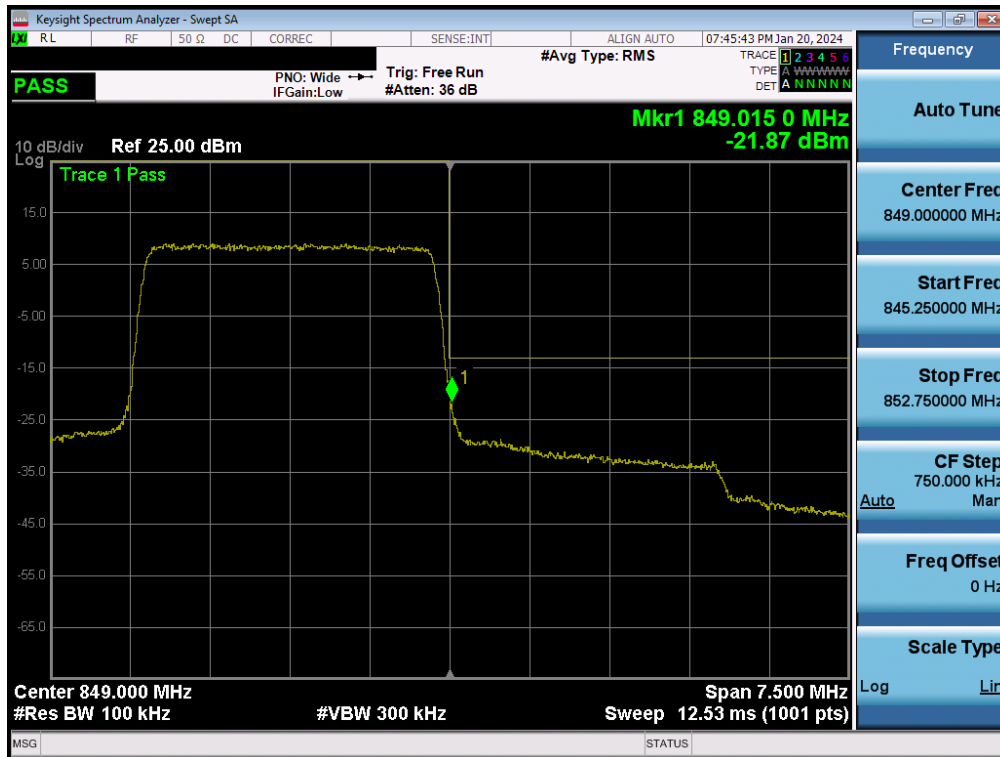
Plot 7-23. Upper Band Edge Plot (LTE Band 5 - 3MHz QPSK – Full RB)
