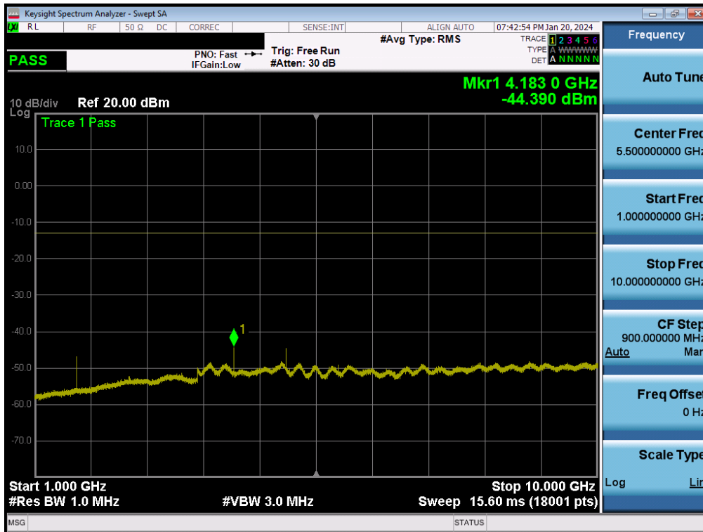
Plot 7-14. Conducted Spurious Plot (LTE Band 5 - 10MHz QPSK - 1 RB - Mid Channel)
