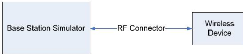
Figure 7-1. Test Instrument & Measurement Setup
