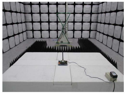
Test Mode: Mode 2: GSM 850\_Idle Mode
