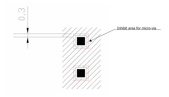
Holes in pad are allowed only for blind holes and not for through holes. Recommendations for PCB pad surfaces:
