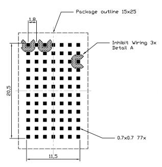
Solder resist pattern Top view
