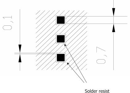
It is not recommended to place via or micro-via not covered by solder resist in an area of 0,3 mm around the pads unless it carries the same signal of the pad itself.
