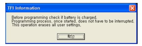
Note: In connection with the HE910V2 modules, charged battery has to be understood that the power supply must not be disconnected during the firmware update.
