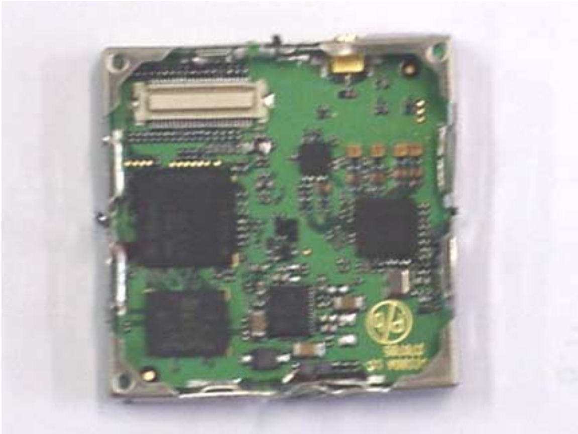
Photo 2. Bottom of EUT with shield removed
