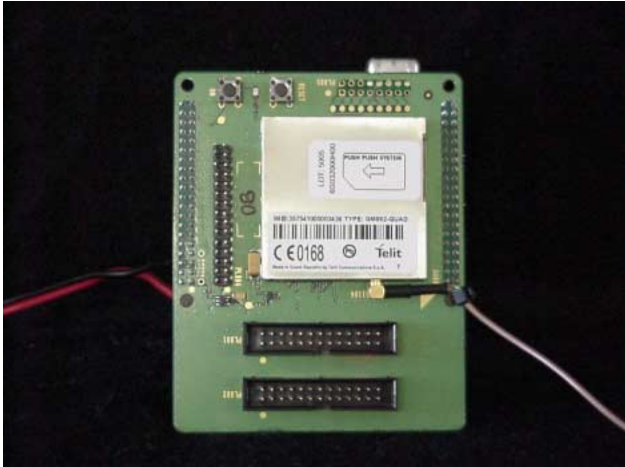
Photo 5. EUT on Test Board with Antenna Cable
