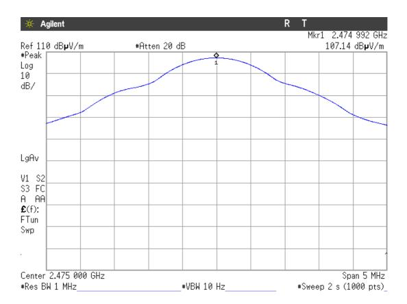
Note: The correction factor is already included in the spectrum analyzer as a transducer factor so that the marker shows directly the field strength level.
