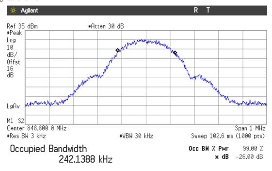
Transmit Freq Error 1.325 kHz x dB Bandwidth 313.104 kHz
