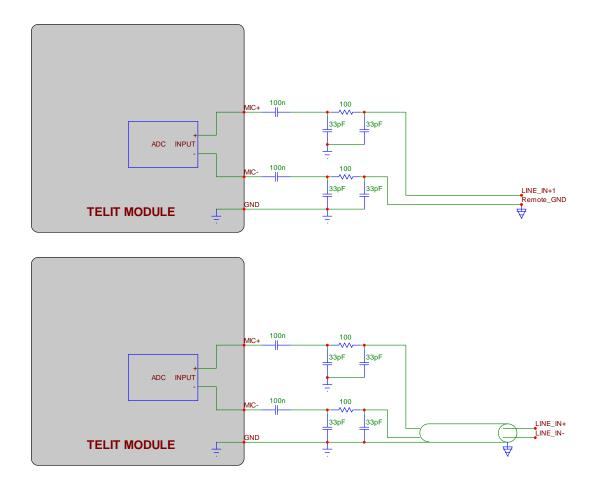
If the audio source is not a mike but a different device, the following connections can be done. Place 100nF capacitor in series with both inputs, so the DC current is blocked.
