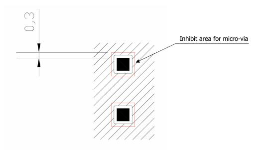
Holes in pad are allowed only for blind holes and not for through holes. When using the hole in pad, we suggest the via filling.
