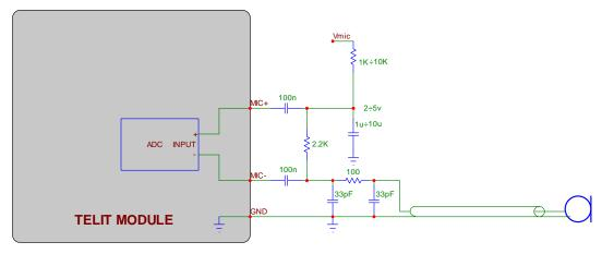
If a "balanced way" is anyway desired, much more care has to be taken to Vmic noise and ground noise; also the 33pF-100Ohm-33pF RF-filter has to be doubled (one each wire).
