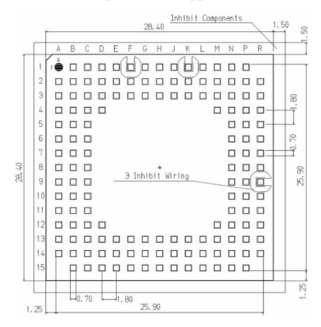
In order to easily rework the GE910 is suggested to consider on the application a 1.5mm Inhibit area around the module.
