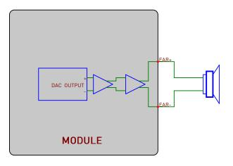
The audio output of the GE910 is balanced, this is helpful to double the level and to reject common mode (click and pop are common mode and therefore rejected). These outputs can drive directly a small loudspeaker with electrical impedance not lower than 80hm.
