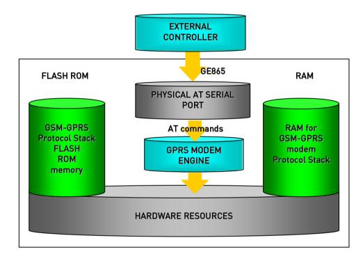
In order to not use any external controller, and further simplify the programming of the sequence of operations, the customer can benefit of these feature already embedded in the GE865:
