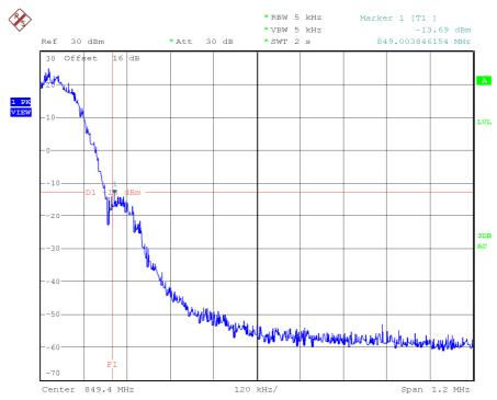
NOTE: The equipment transmits at the maximum output power (PCL= 5).
