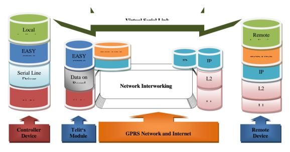
This particular implementation allows to the devices interfacing to the modules the use of the GPRS and Internet packet service without the need to have an internal TCP/IP stack since this function is embedded in the module.
