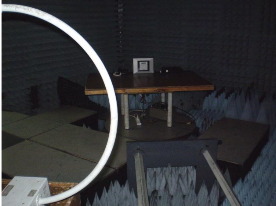
Photograph No.1 Setup for spurious emission field strength measurements of PowerMax Pro containing GE864 (GSM) module in anechoic chamber below 30 MHz
