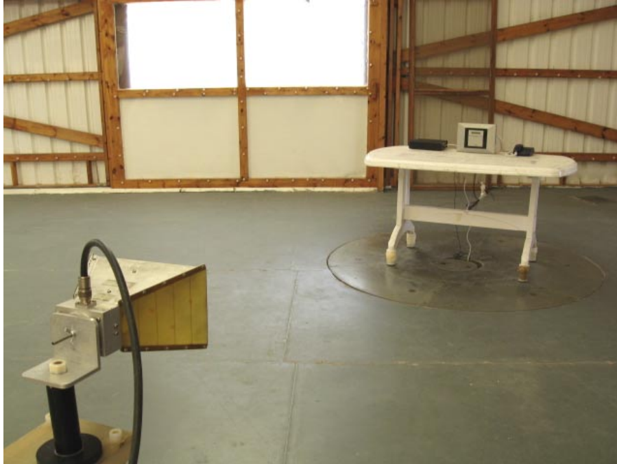
Photograph No.4 Setup for spurious emission field strength measurements at the OATS above 1000 MHz range
