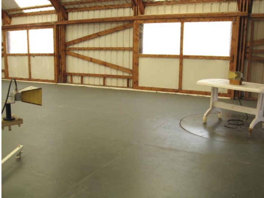
Photograph No.6 Setup for substitution peak output power measurements in 1850 – 1910 MHz range
