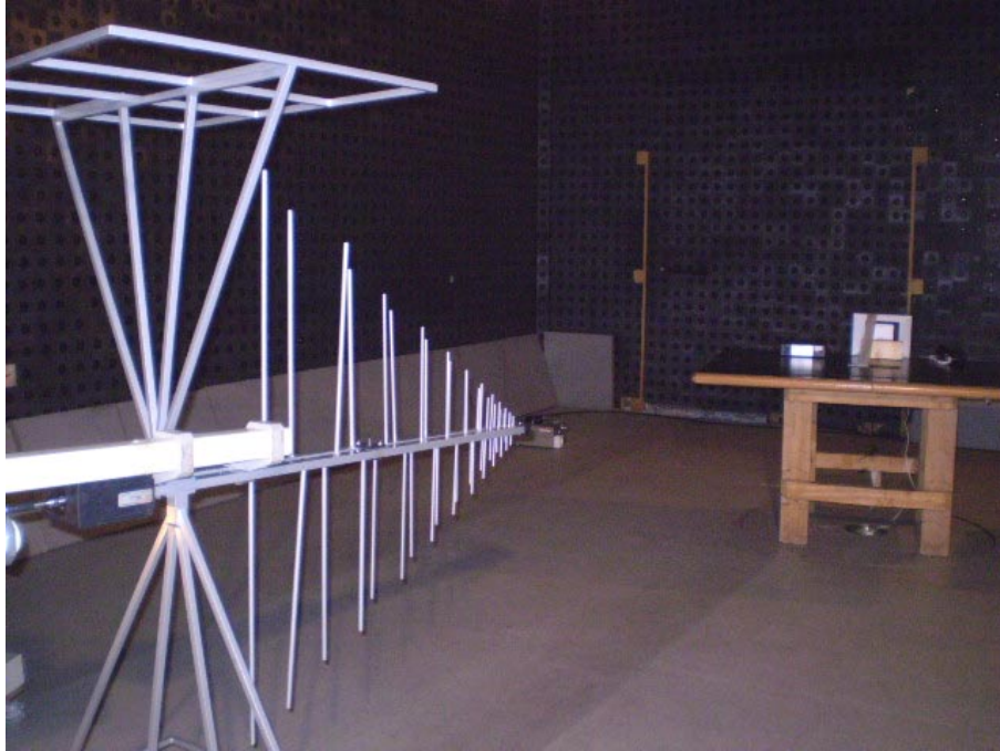
Photograph No.2 Setup for carrier and spurious emission field strength measurements of PowerMax Pro containing GE864 (GSM) module in anechoic chamber in 30 – 1000 MHz range
