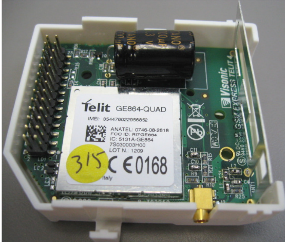
Photograph No.3 GSM modem second side internal view
