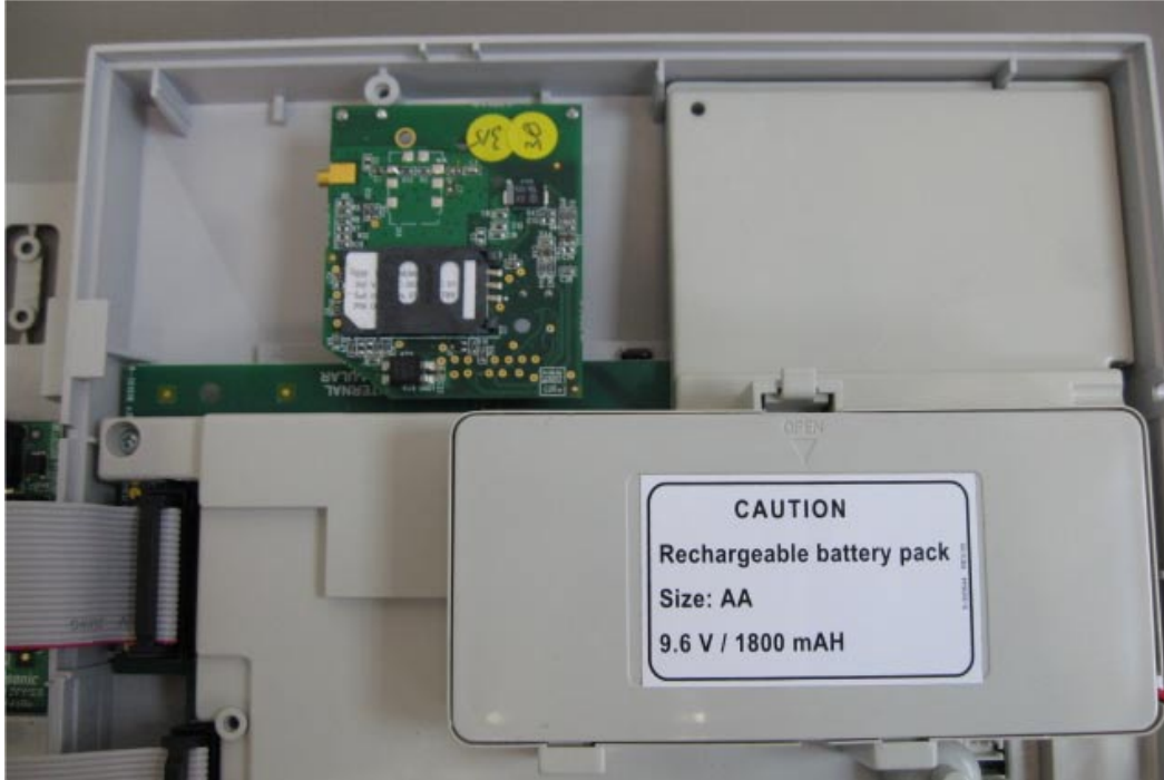
Photograph No.2 GSM modem without case located in PowerMax Pro
