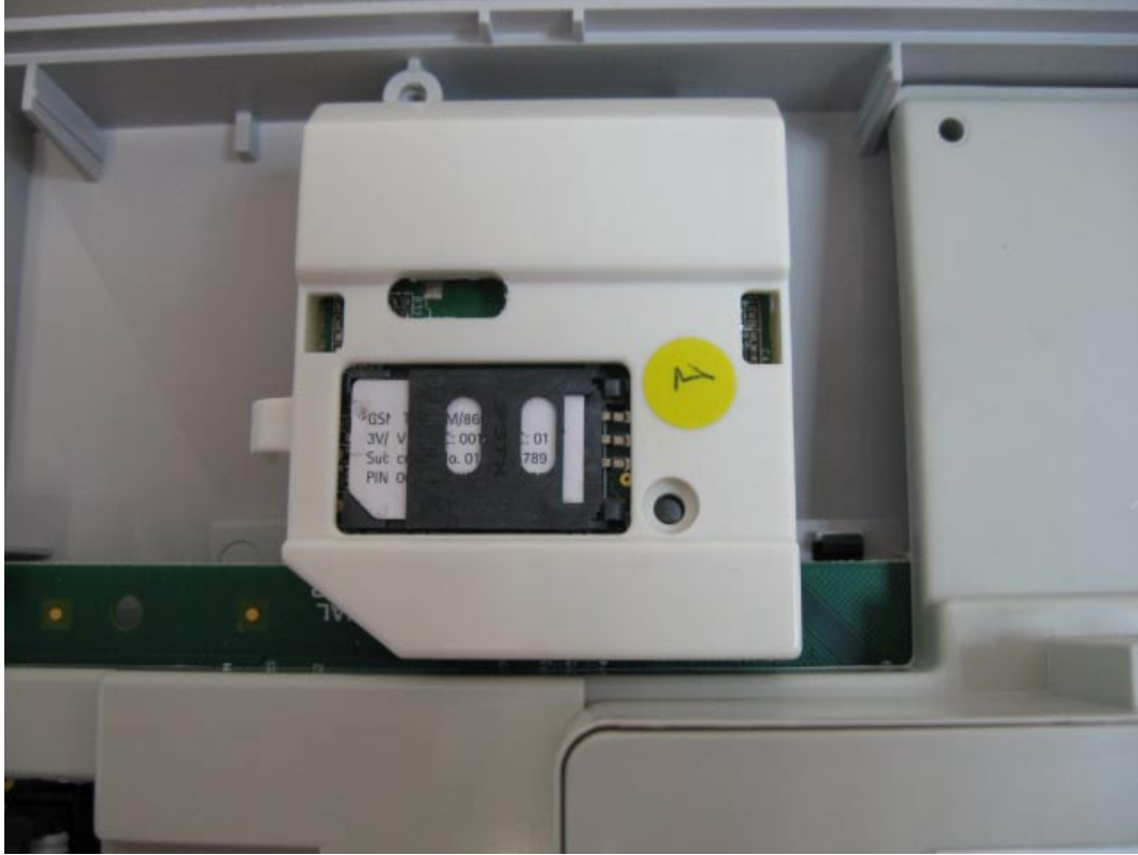
Photograph No.1 GSM modem located in PowerMax Pro
