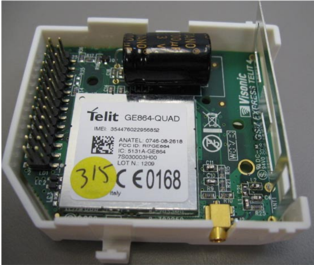
Photograph No.3 GSM modem rear side view
