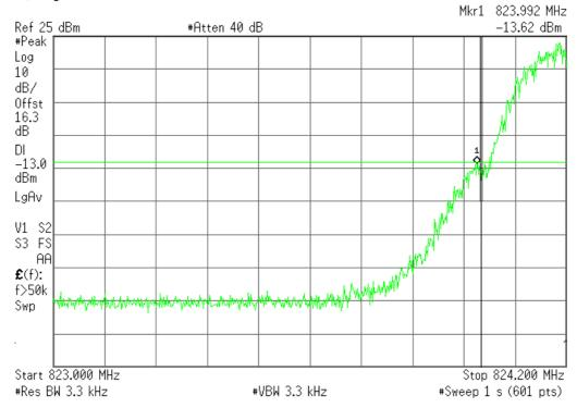
NOTE: The equipment transmits at the maximum output power (PCL= 5).
