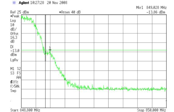
NOTE: The equipment transmits at the maximum output power (PCL= 5).
