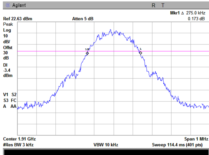
Plot 8.2.6 Occupied bandwidth test result at high frequency
