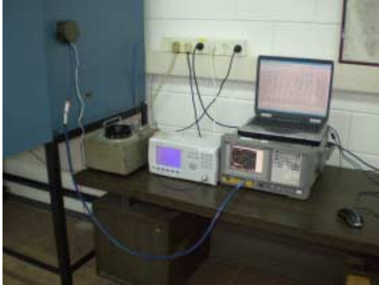
Photograph No.10 Frequency stability measurement set up
