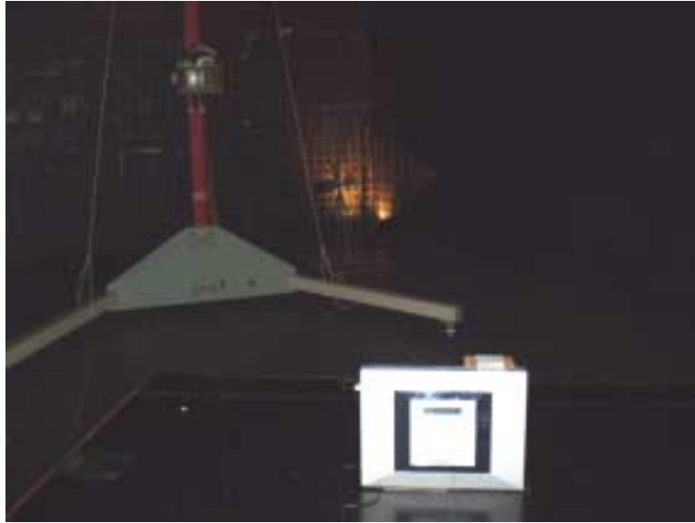
Photograph No.1 Setup for carrier field strength measurements of PowerMax Pro containing GE863 (GSM) module
