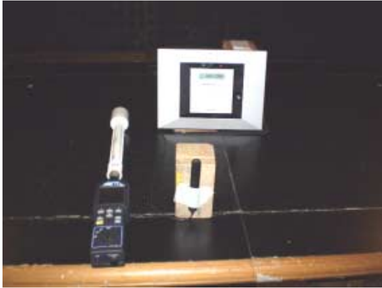
Photograph No.8 Maximum permissible exposure (MPE) measurement set up, PowerMax Pro containing GE863 (GSM) module
