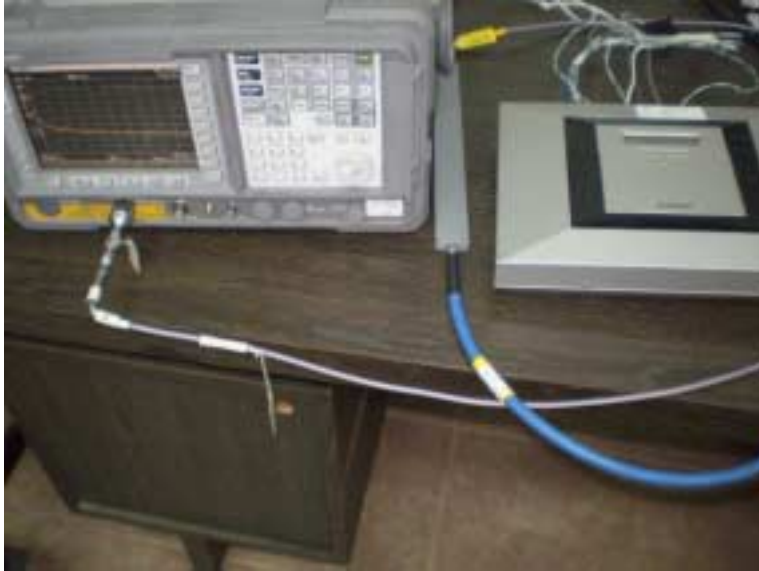
Photograph No.7 Occupied bandwidth and conducted spurious emission measurements setup
