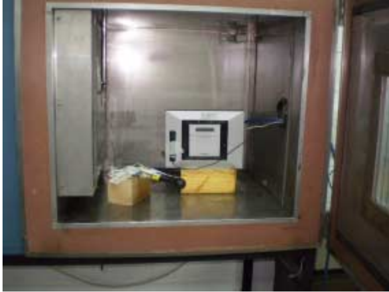
Photograph No.9 Frequency stability measurement set up
