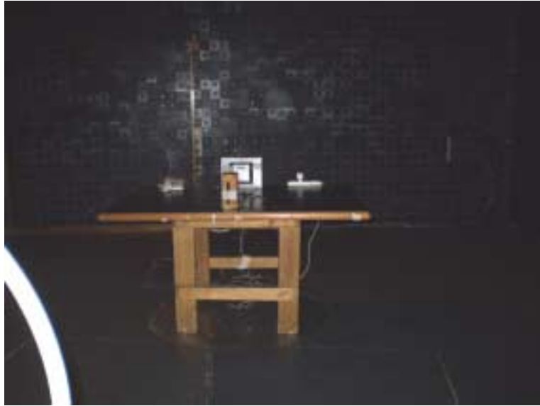
Photograph No.4 Setup for spurious emission field strength measurements in anechoic chamber below 30 MHz
