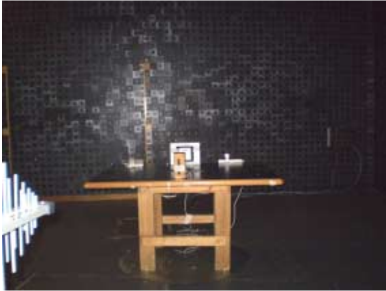
Photograph No.5 Setup for spurious emission field strength measurements in anechoic chamber in 30 – 1000 MHz range
