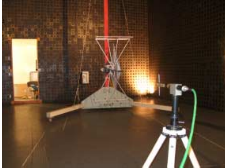
Photograph No.2 Setup for substitution peak output power measurements in 824 – 849 MHz range
