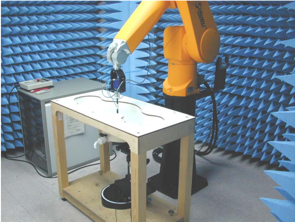
Fig.1 Photograph of the SAR measurement System
