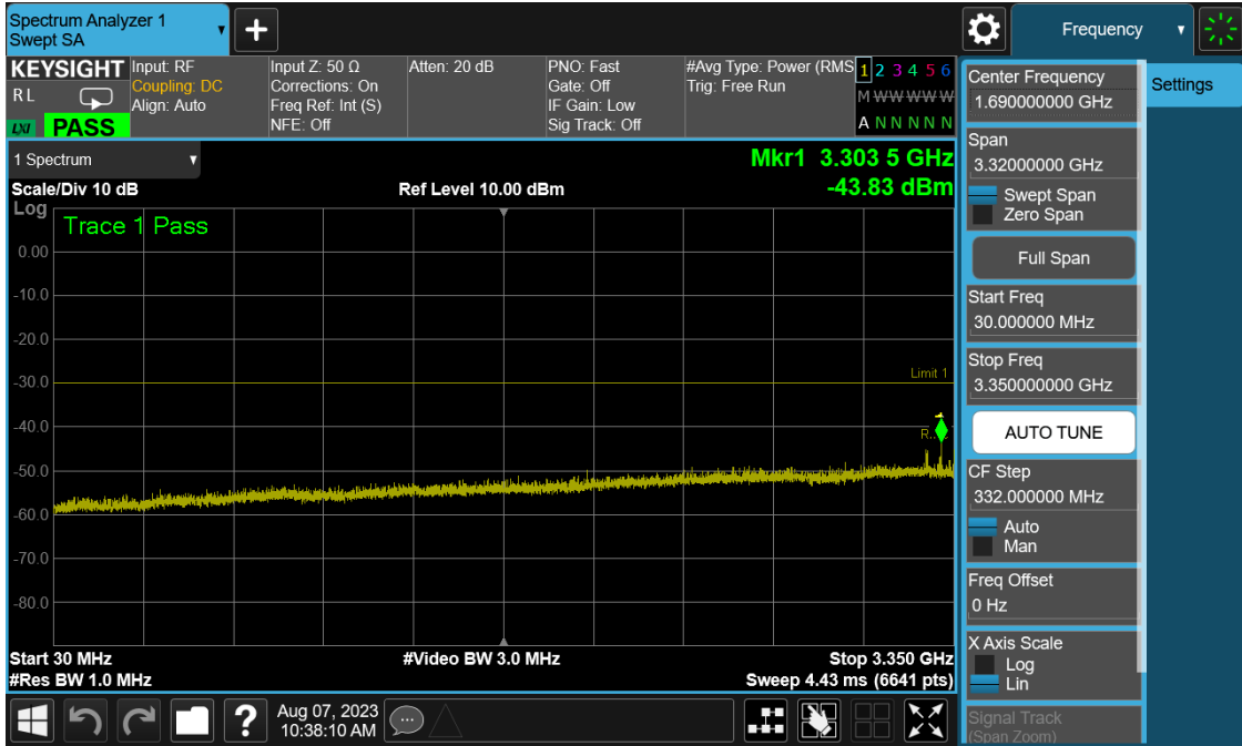
Plot 7-35. Conducted Spurious Plot (NR Band n78 - 10MHz QPSK - Low Channel)
