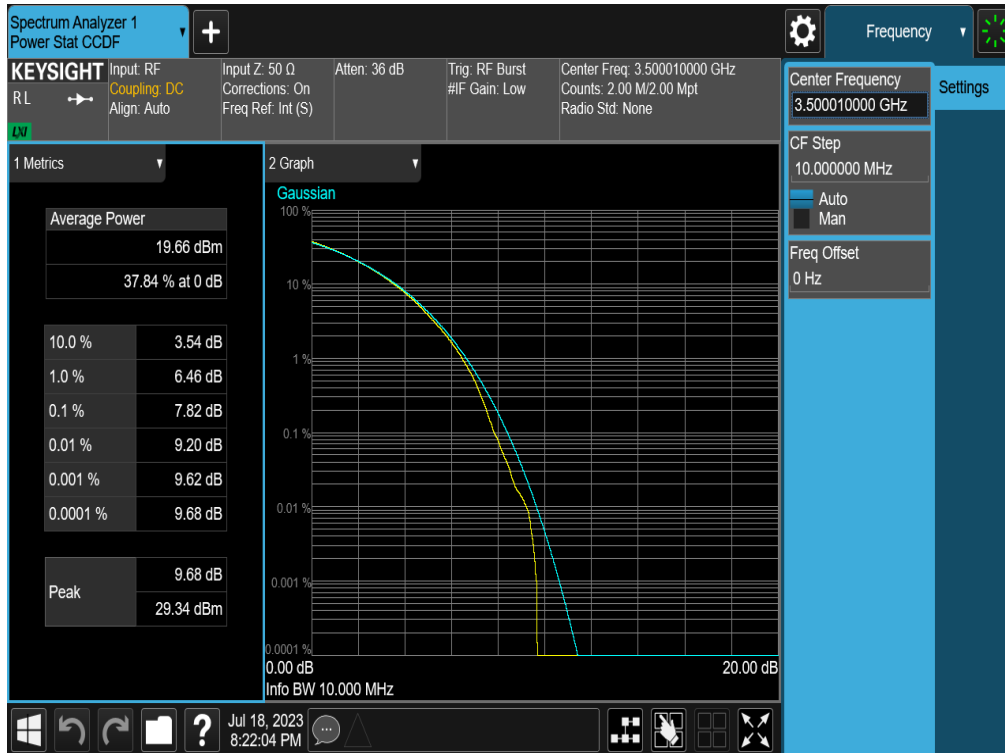
Plot 7-51. PAR Plot (NR Band n78 - 10MHz CP-OFDM 256-QAM- Full RB)
