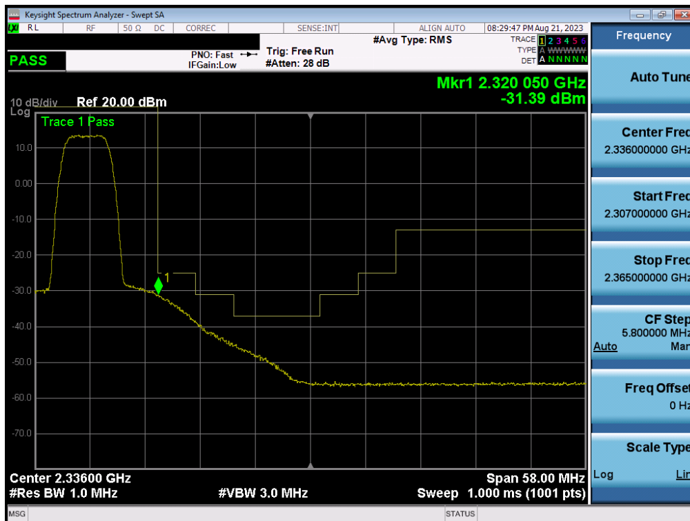
Plot 7-16. Extended Upper Band Edge Plot (NR Band n30 - 5MHz QPSK – Full RB)
