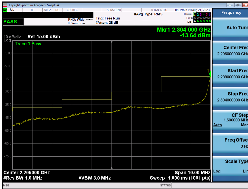
Plot 7-14. Extended Lower Band Edge Plot (NR Band n30 - 5MHz QPSK – Full RB - Ant1)
