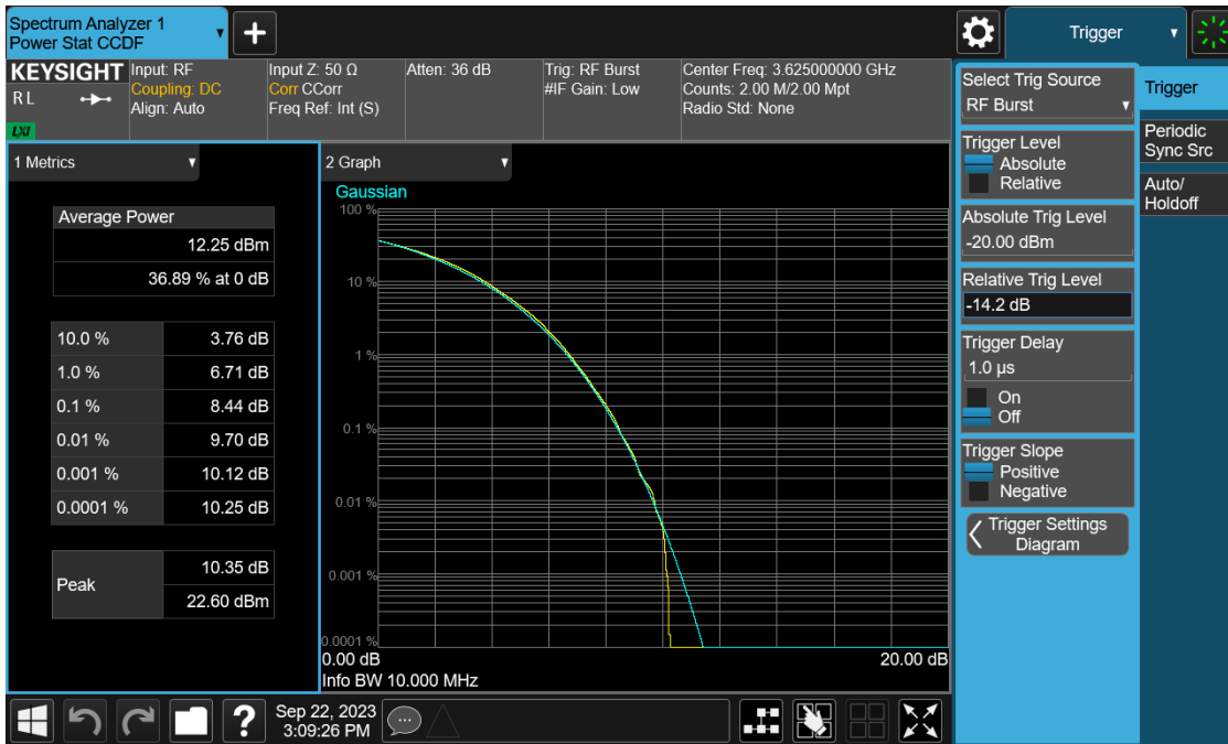
Plot 7-58. PAR Plot (NR Band n78 - 10MHz CP-OFDM 256-QAM– Full RB)
