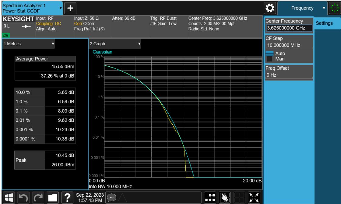
Plot 7-56. PAR Plot (NR Band n78 - 10MHz CP-OFDM 256-QAM- Full RB)
