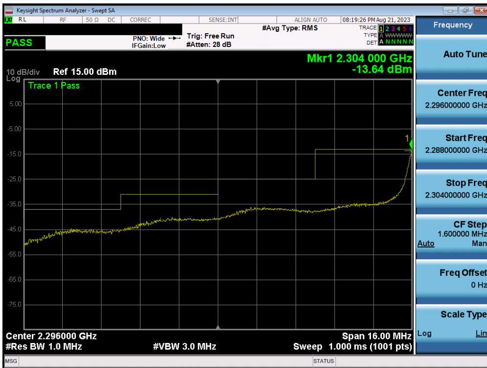
Plot 7-14. Extended Lower Band Edge Plot (NR Band n30 - 5MHz QPSK – Full RB - Ant1)
