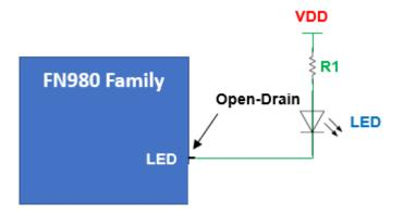
R1 and VDD determine the brightness of LED and forward current.
