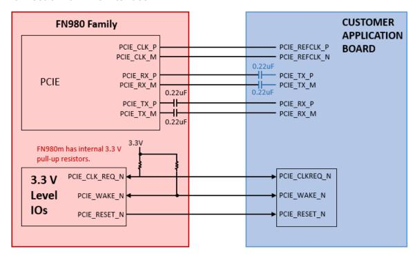
\*CUSTOMER: Need to series capacitor (0.22uF) at PCIE\_TX\_P/M Lines
